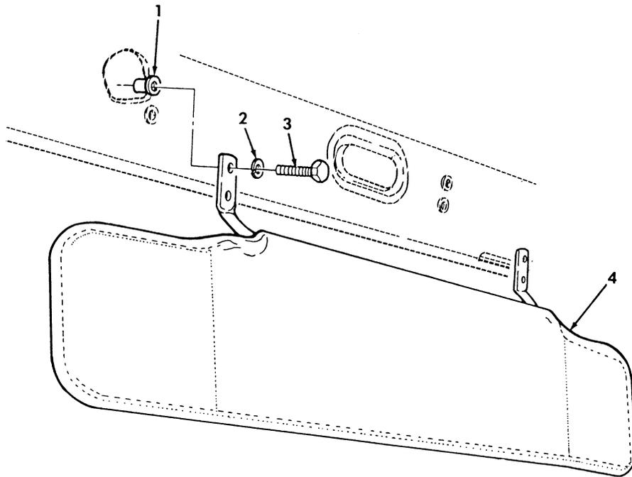
Figure 352. Sun Visor Assembly and Mounting Hardware.
