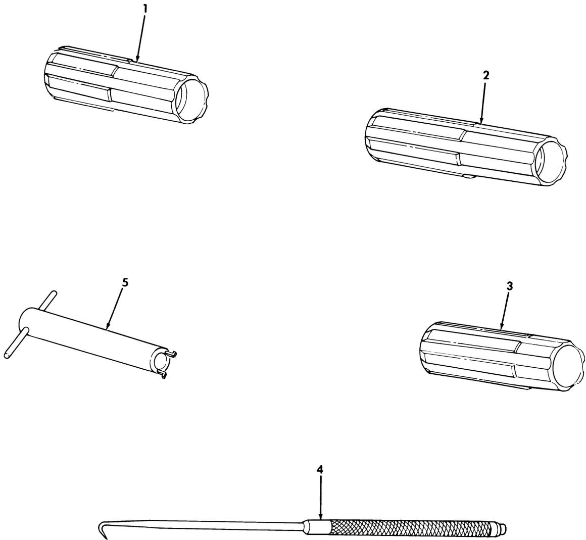
*Figure 508. Special Tools, Air Conditioner Compressor.*
