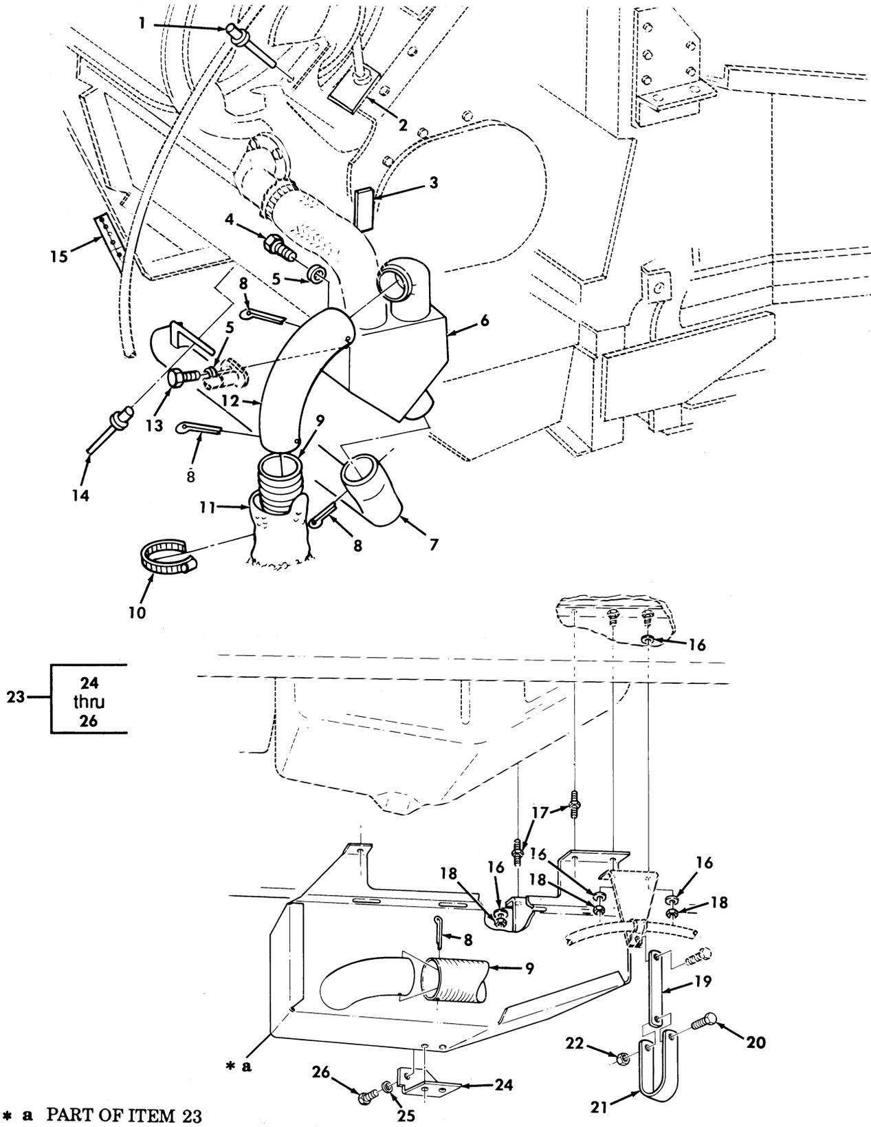
Figure 365. Arctic Kit, Pan Cover and Heater Tube.
