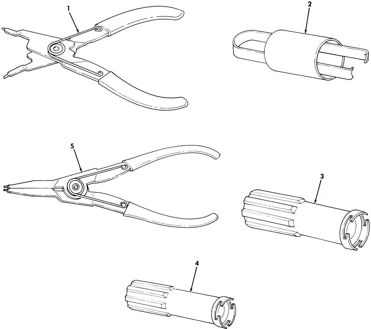
Figure 507. Special Tools, Air Conditioner Compressor.
