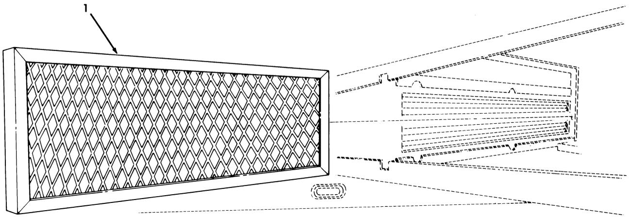
*Figure 344. Air Intake Filter, M996 and M996A1 Ambulance.*
