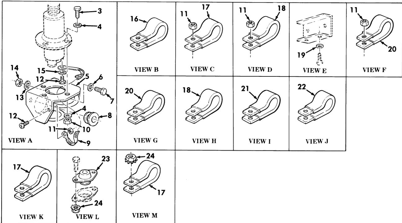
Figure 428. Communications Kit, Radio Cables, (3) AN/VRC-46.
