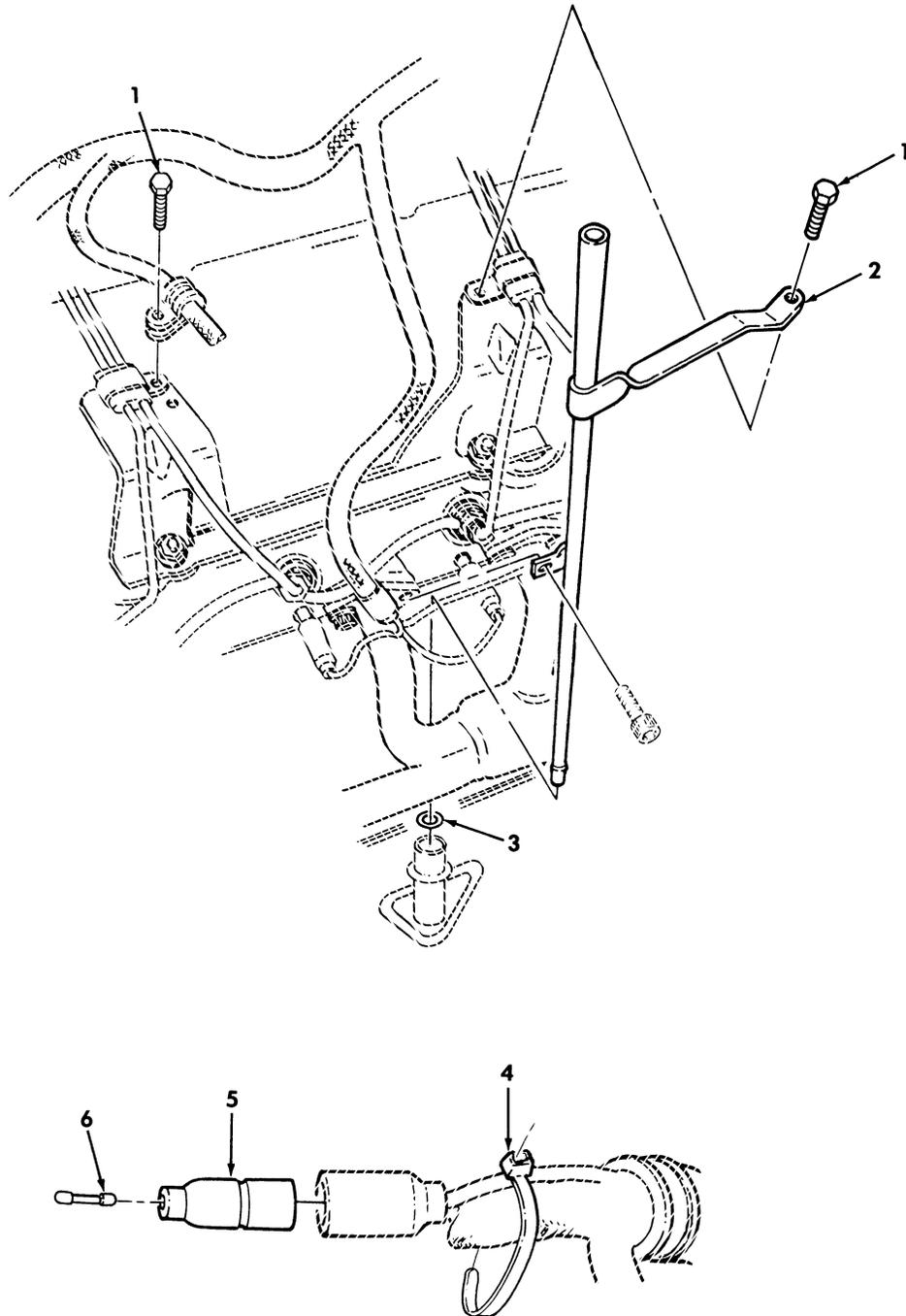
Figure 479. Dipstick and Dummy Connector Plug-400 AMP Alternator Kit.
