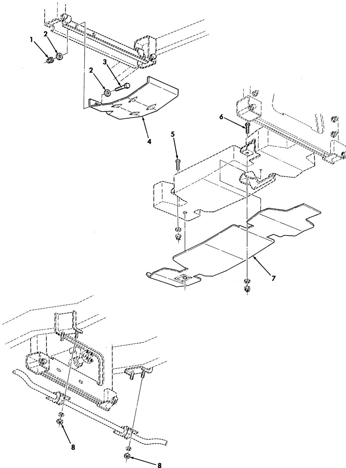
Figure 464. Underbody Protection Kit, Transfer Case, Fuel Tank Shields, and Sway Bar Link Nuts.
