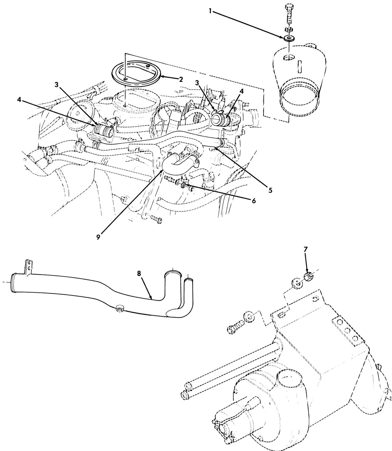
Figure 364. Arctic Kit, Fuel Injection Pump, Engine Gaskets, and CDR Tube.
