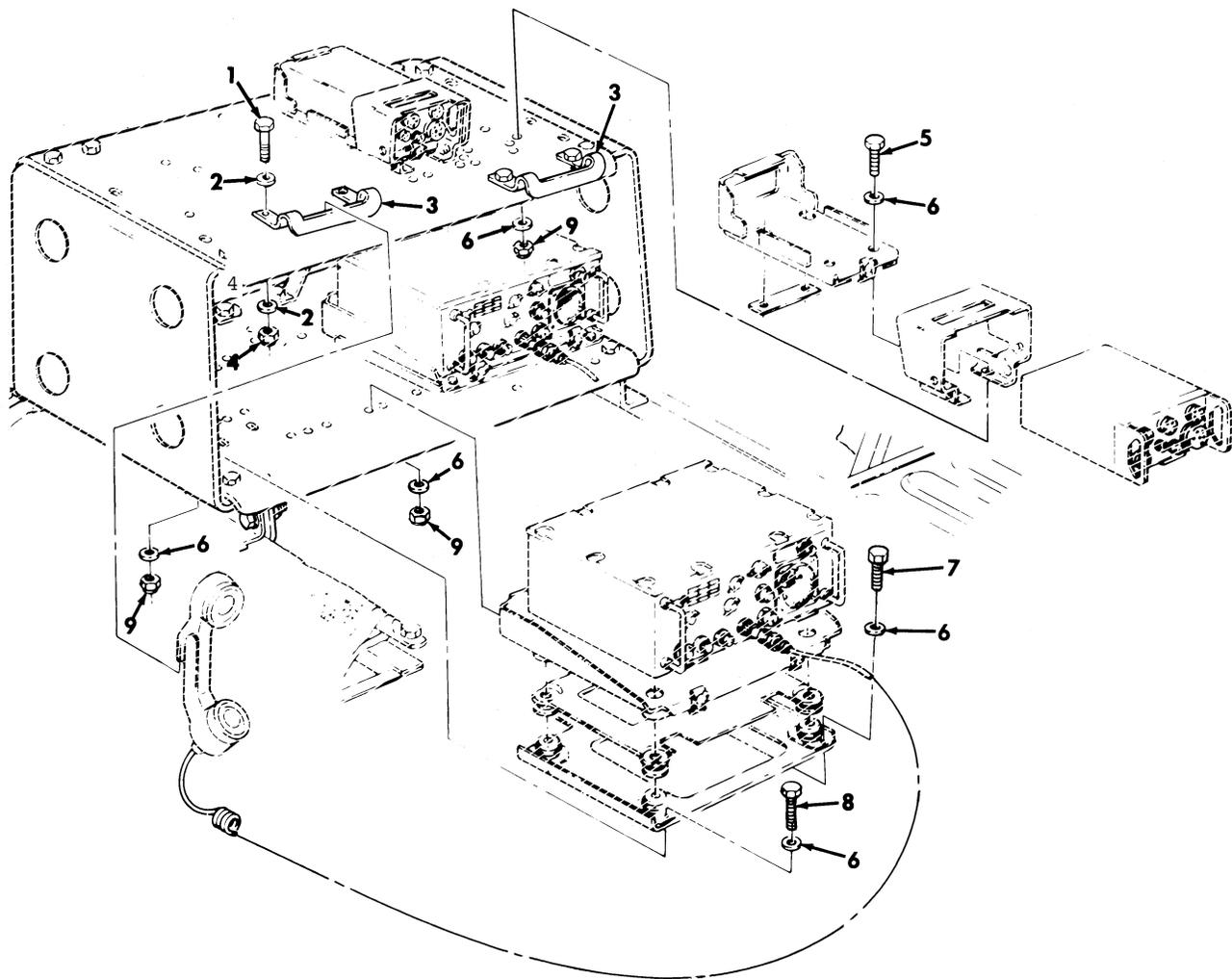
Figure 419. Communications Kit, Radio Rack Assembly Mounting Hardware, (2) AN/VRC-46.
