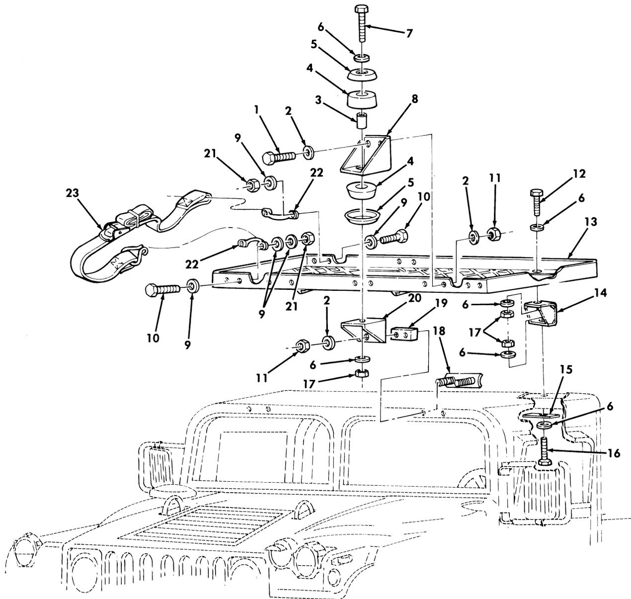
Figure 440. Kit, Camouflage Rack and Stowage Rack Assembly.
