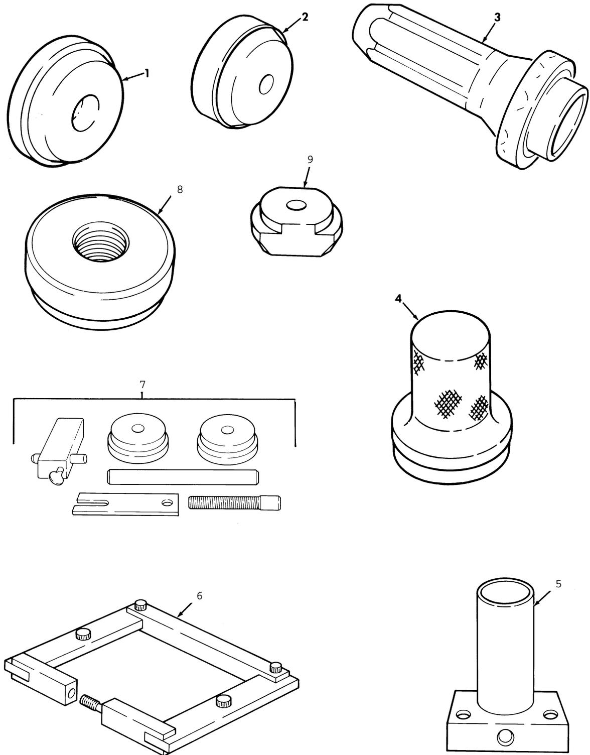
Figure 502. Special Tools, Axle Differential.
