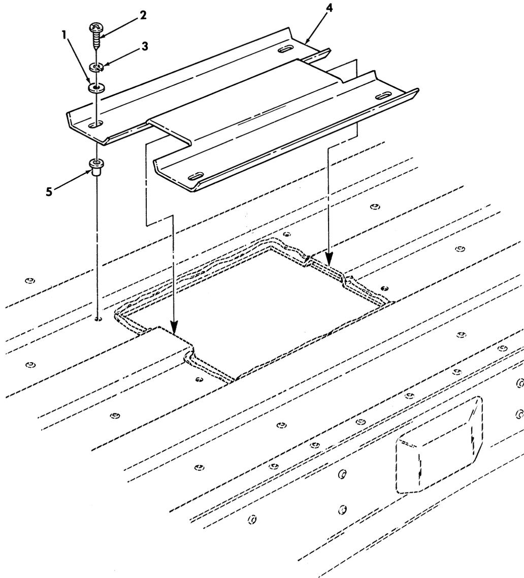
Figure 465. Cover, Access Cargo Floor Modification Kit.
