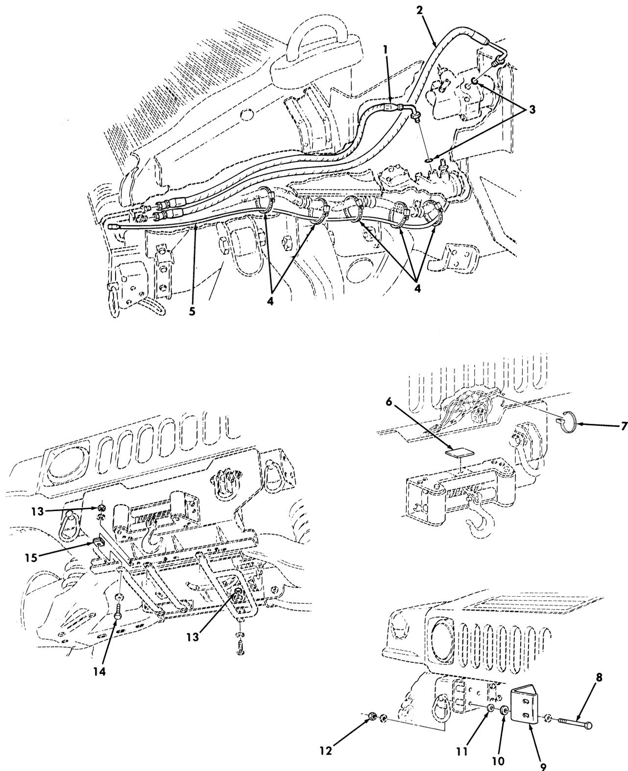
Figure 470. 10,500 Lb Hydraulic Winch Accessory Kit.
