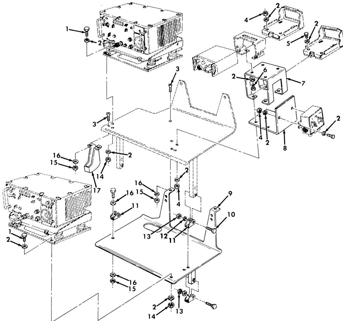
Figure 415. Communications Kit, Radio Rack Assembly, AN/VRC-49, and (2) TSEC/KY-57 Assemblies.
