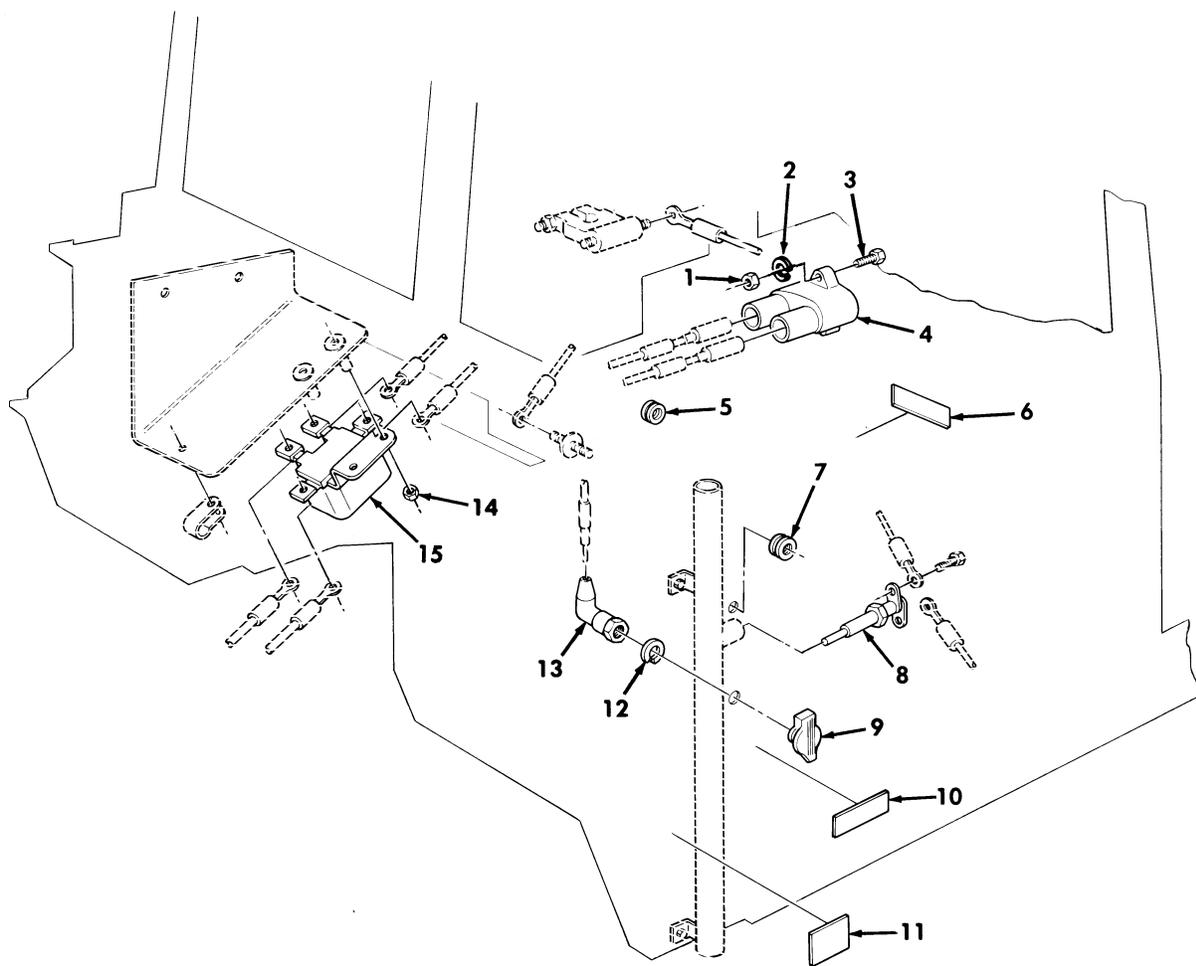
Figure 380. Swingfire Heater Kit, Circuit Breaker and Related Parts.
