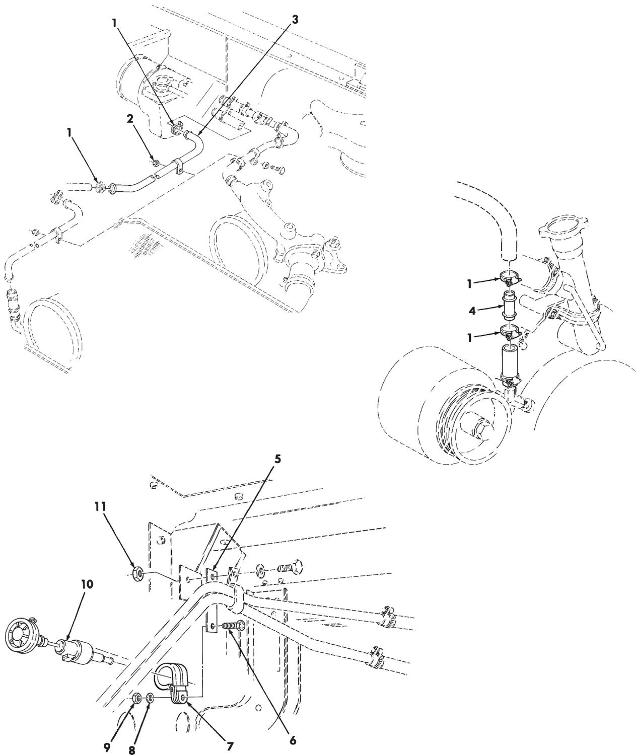
Figure 397E. Crew and Engine Compartment Heater Fuel Pump, Lines, and Mounting Hardware.
