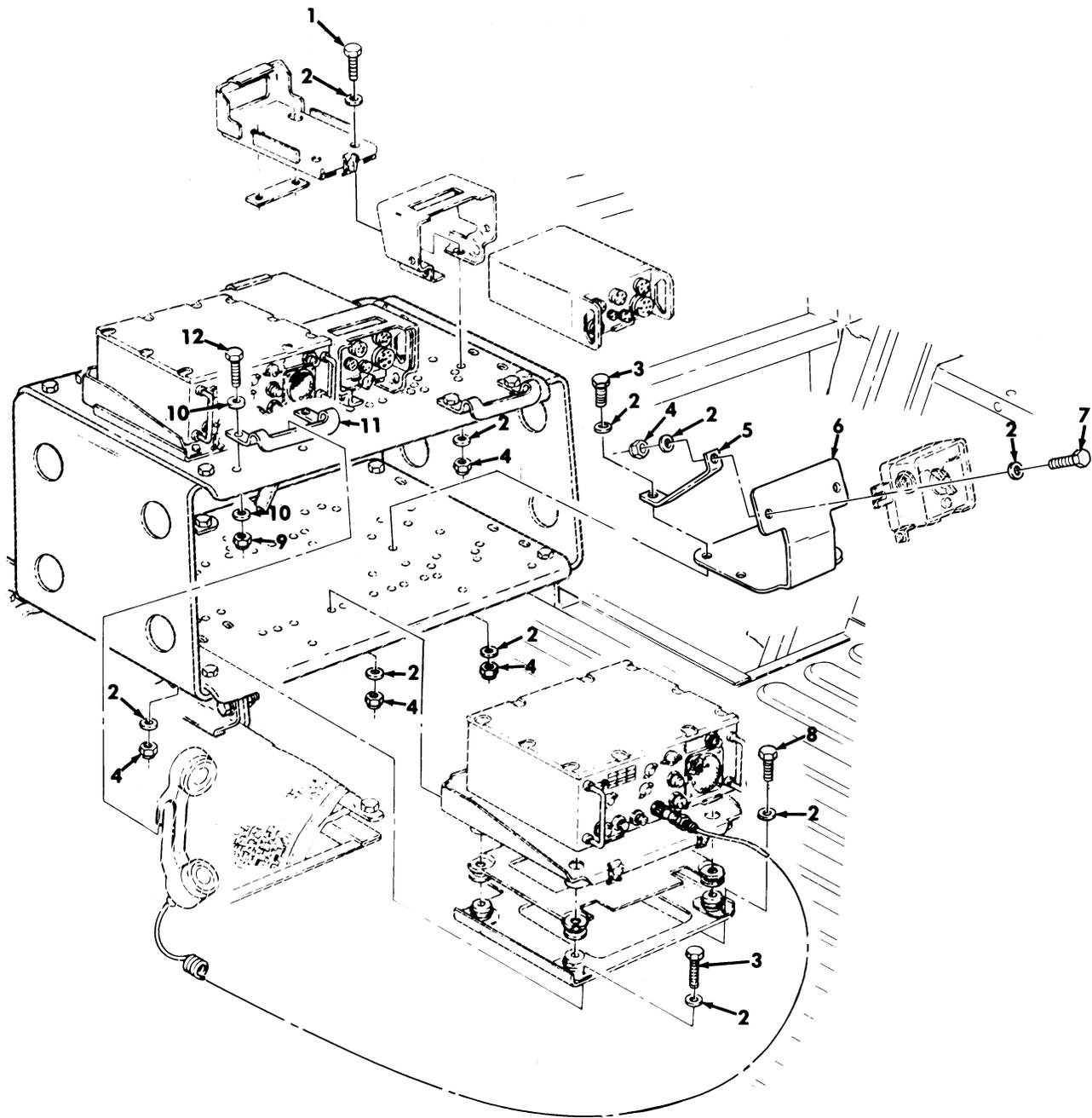
Figure 423. Communications Kit, Radio Rack Assembly Mounting Hardware, AN/VRC-49.
