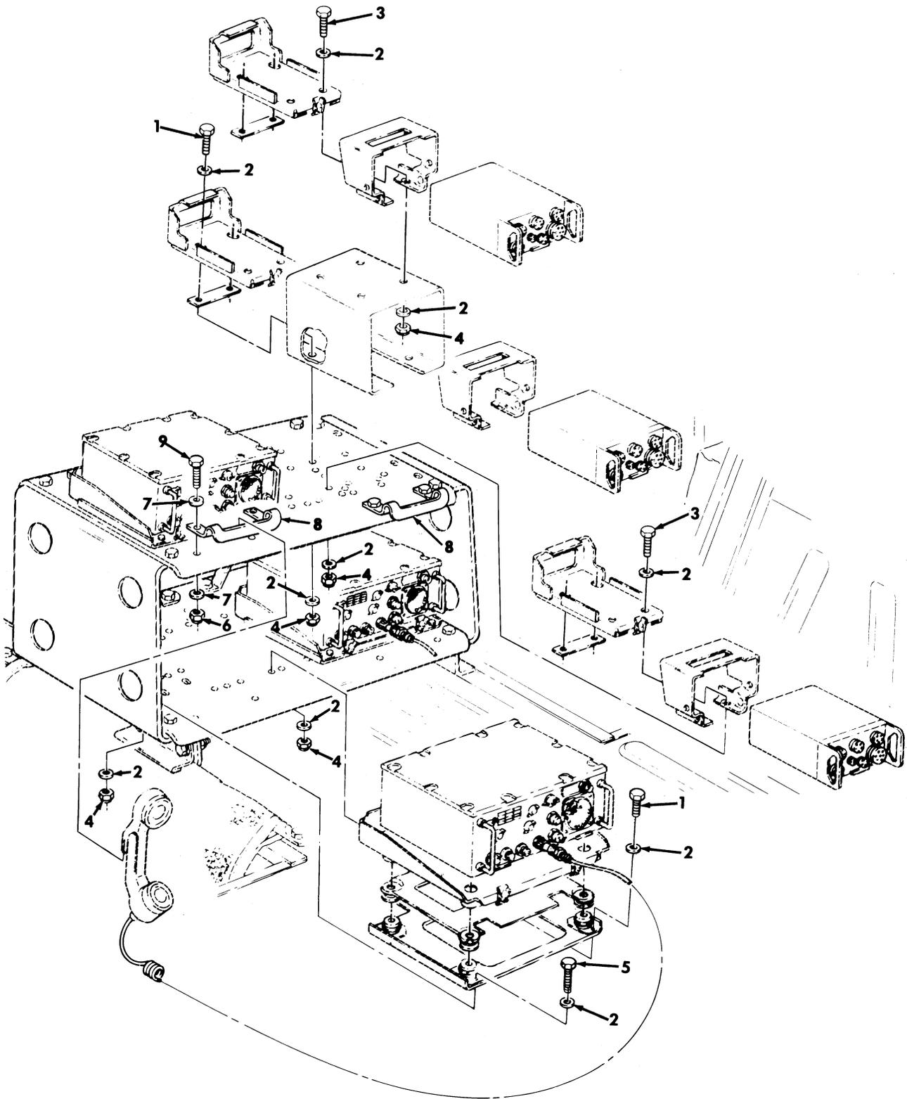
Figure 420. Communications Kit, Radio Rack Assembly Mounting Hardware, (3) AN/VRC-46.
