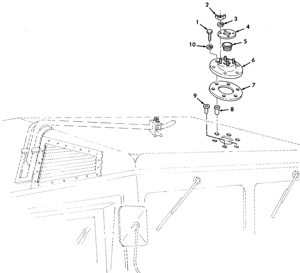
Figure 340. Antenna Mount and Mounting Hardware, M996 and M996A1 Ambulance.
