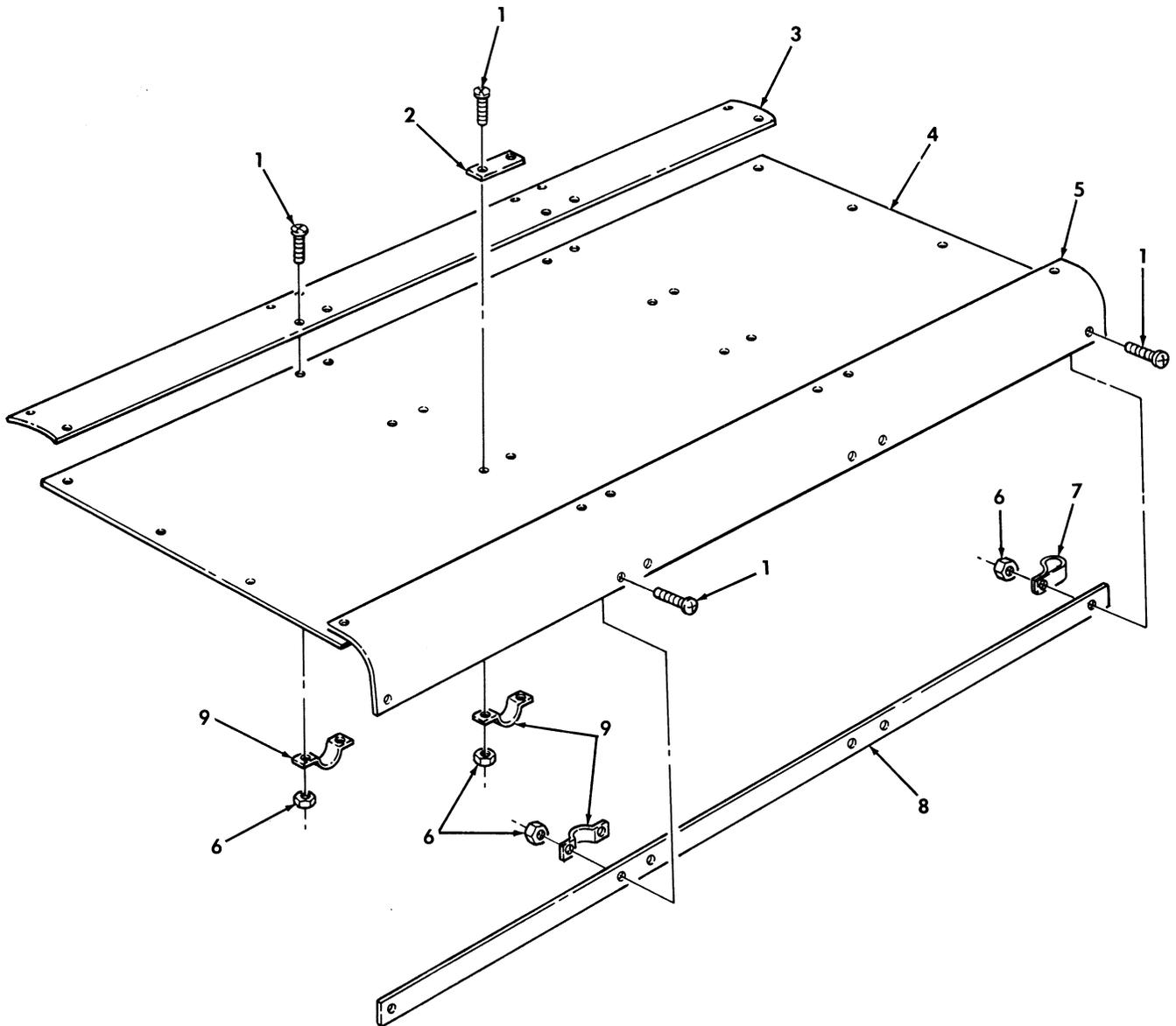
Figure 391. Top Plate Support and Attaching Hardware.
