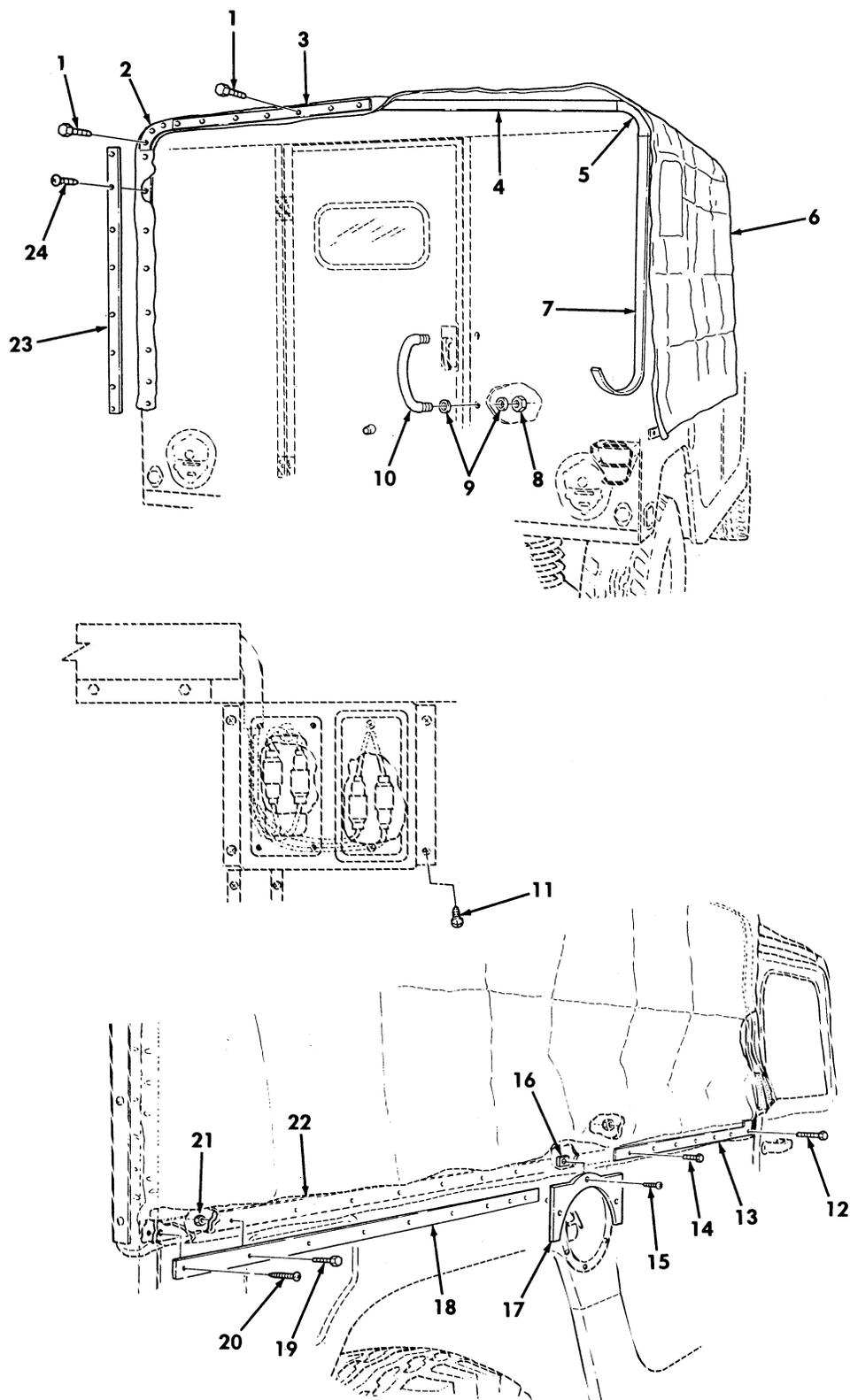
Figure 395. Top Cover Assembly and Mounting Hardware.
