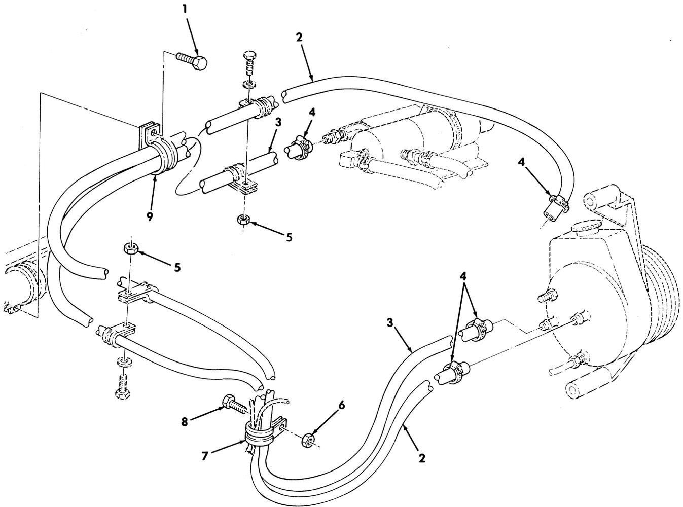
Figure 477. Power Steering Pump Hoses-400 AMP Alternator Kit.
