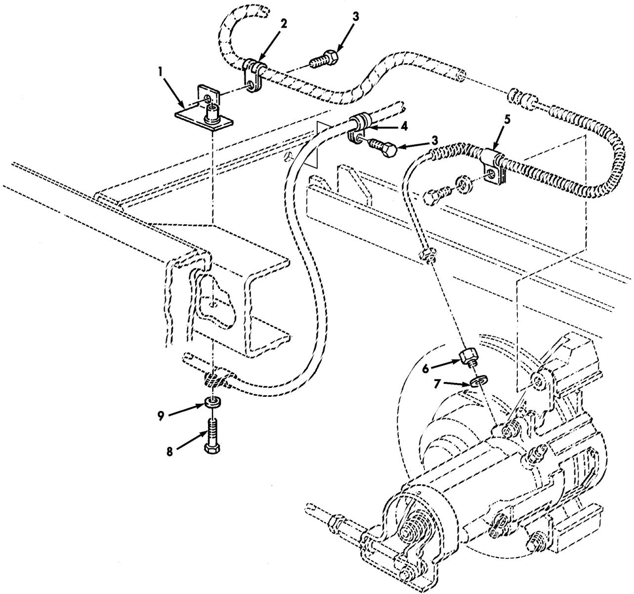
Figure 487D. Flexible Brake Line Kit.
