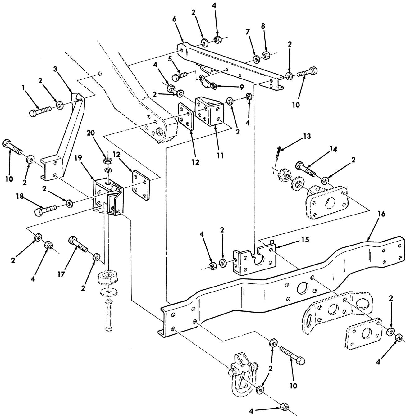
Figure 442. Kit, Prime Mover, Lt. Howitzer, 105 MM L119, Rear Bumper.
