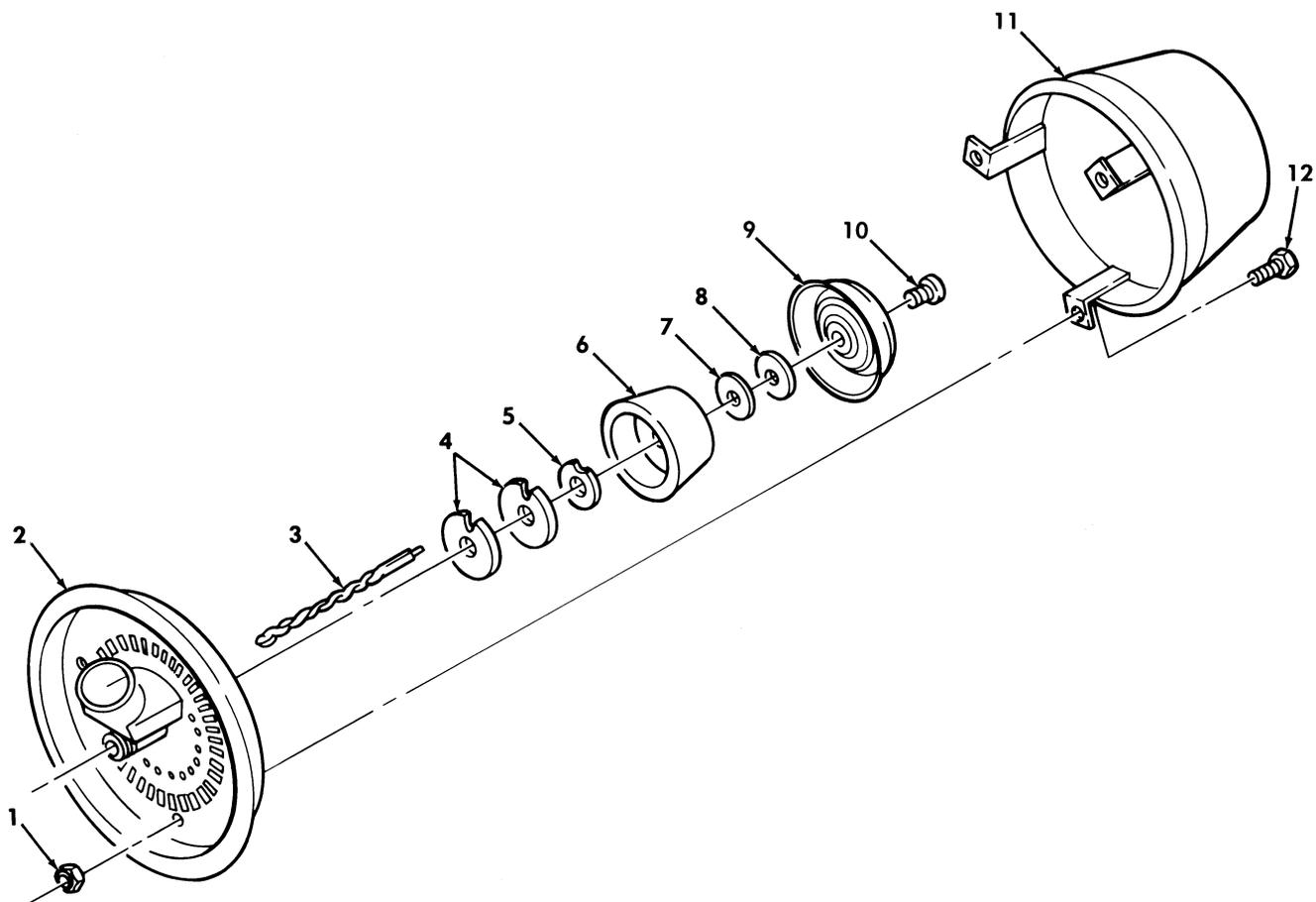
Figure 350. Burner Assembly, B-Model, M996, M996A1, M997, M997A1, and M997A2 Ambulance.
