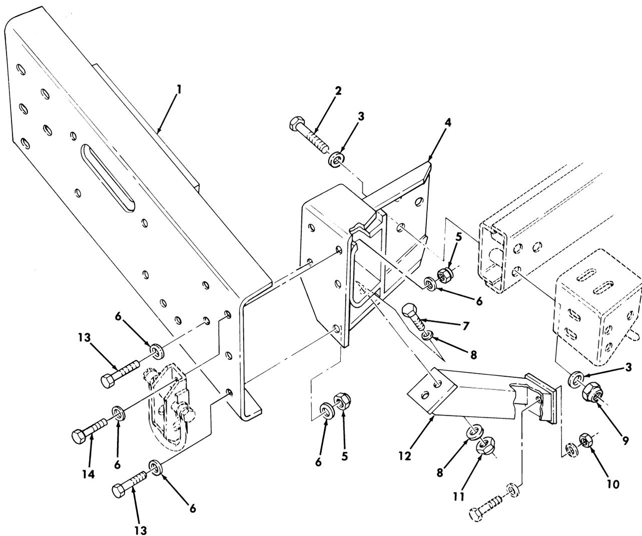
Figure 441. Kit, Prime Mover, Lt. Howitzer, 105 MM L119, Front Bumper.
