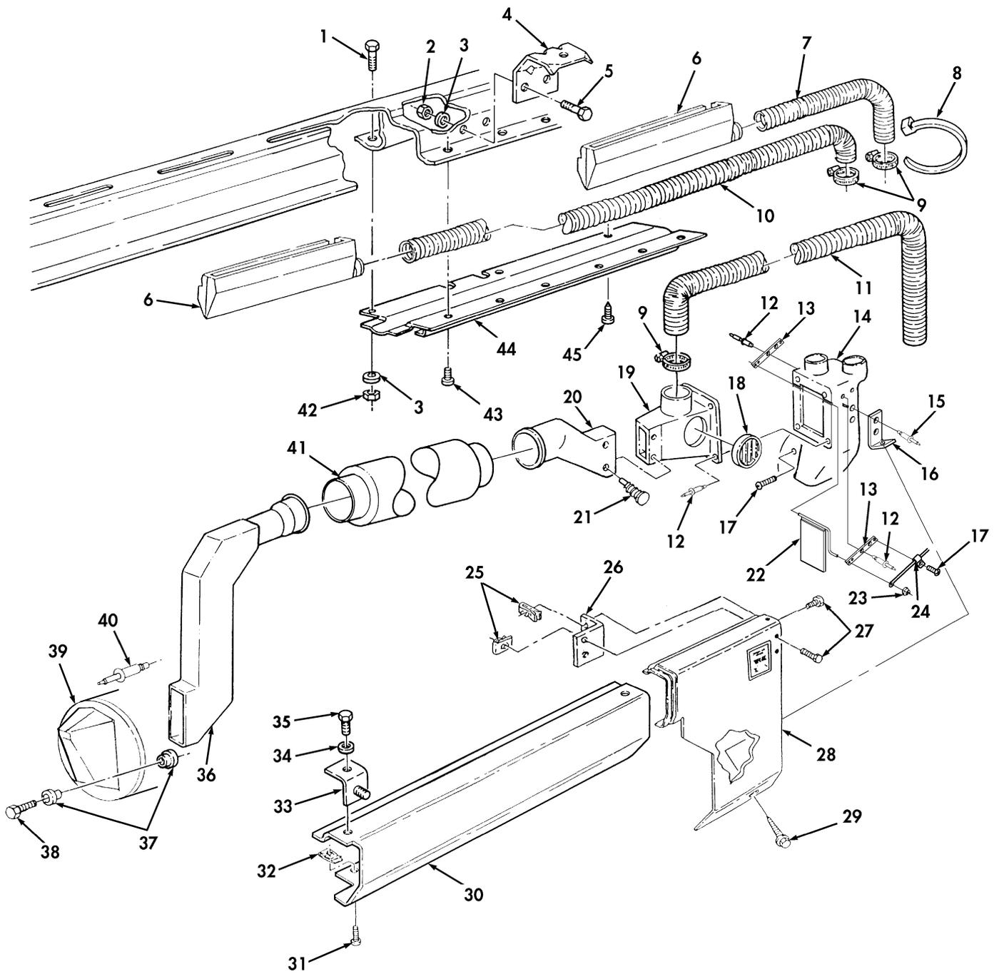
Figure 332. A2 Diverter Assembly, Defroster, Heater Ducting, and Radio Brackets.
