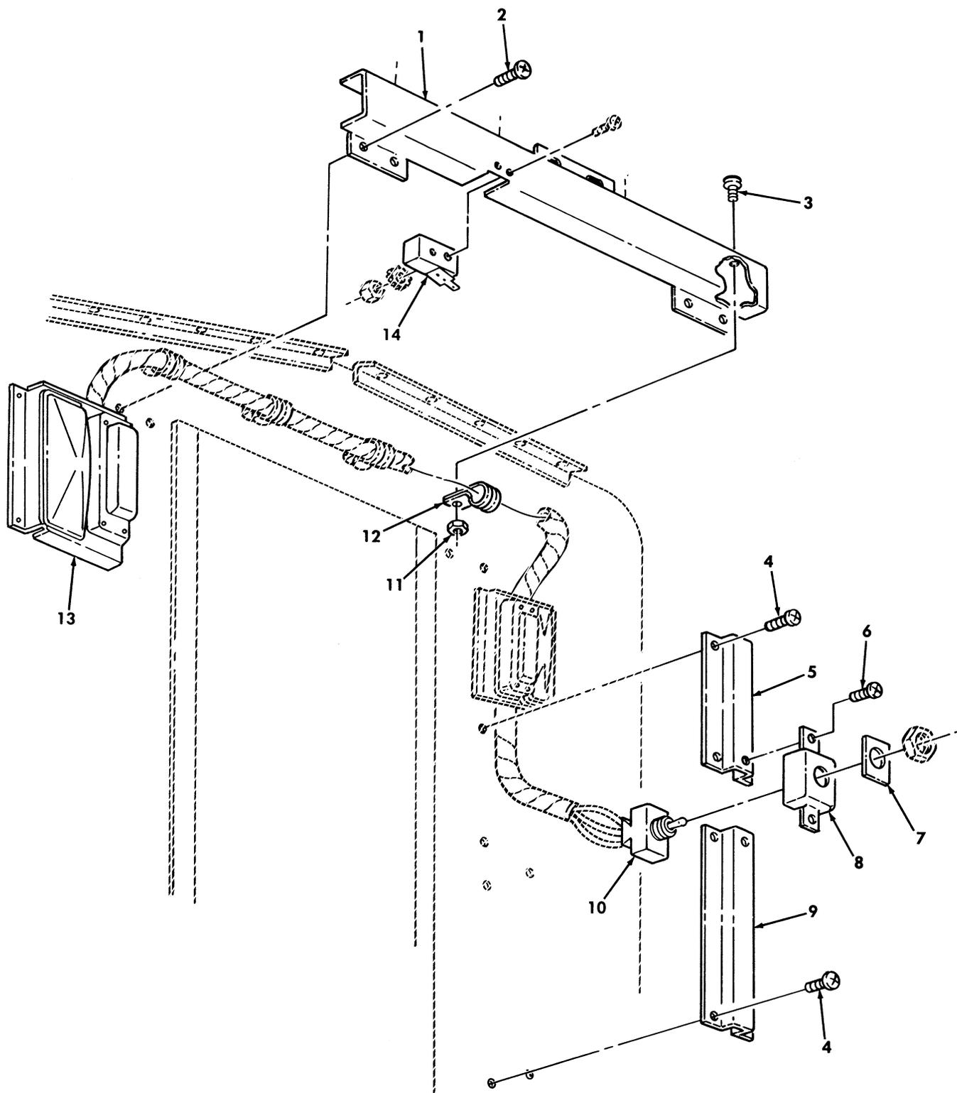
Figure 396. Wiring Harness Channel and Hardware.
