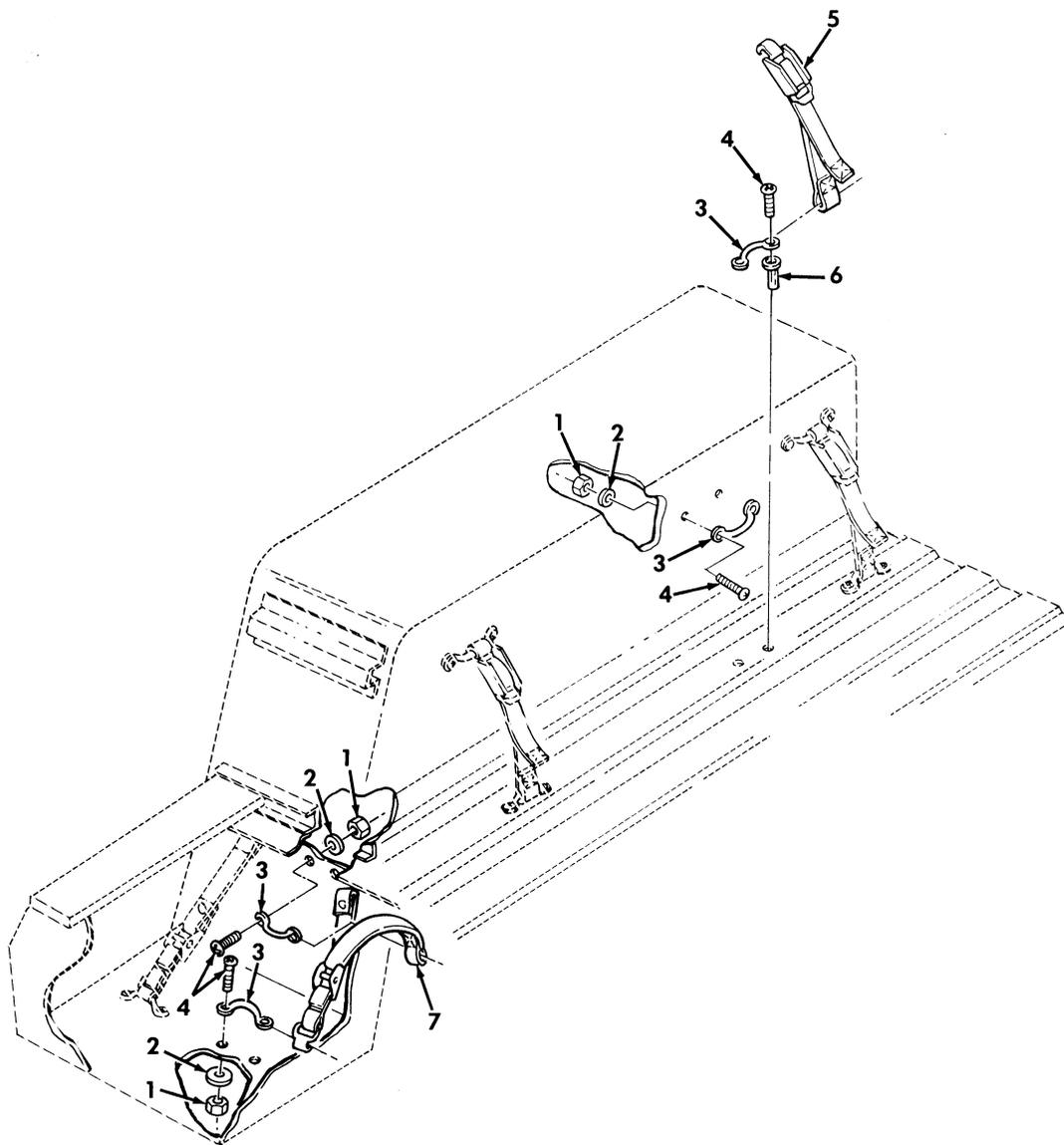
Figure 450. Kit, Prime Mover, Lt. Howitzer, 105 MM L119, Aiming Post and Cable Reel Stowage.
