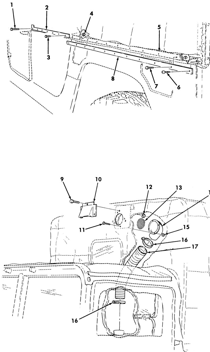
Figure 393. Mounting Plates and Ventilator Exhaust Ducting.
