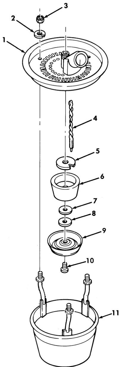
Figure 351. Burner Assembly, A-Model, M997, M997A1, and M997A2 Ambulance.
