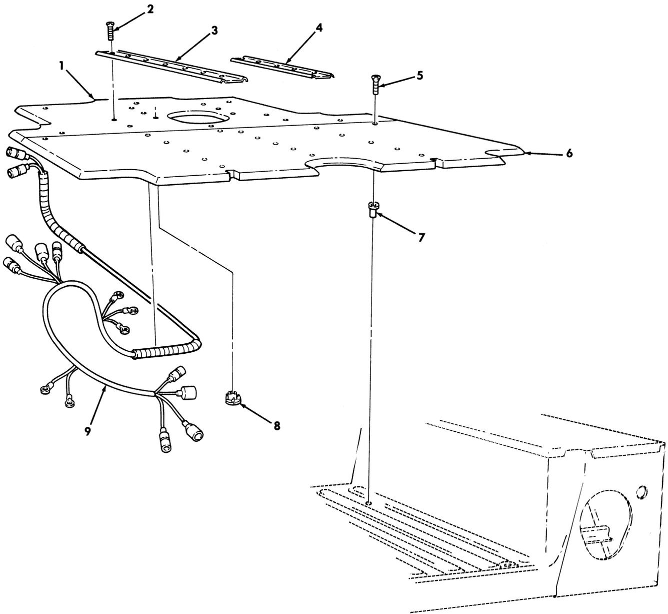
Figure 383. Cargo Floor Cover and Harness Assembly.
