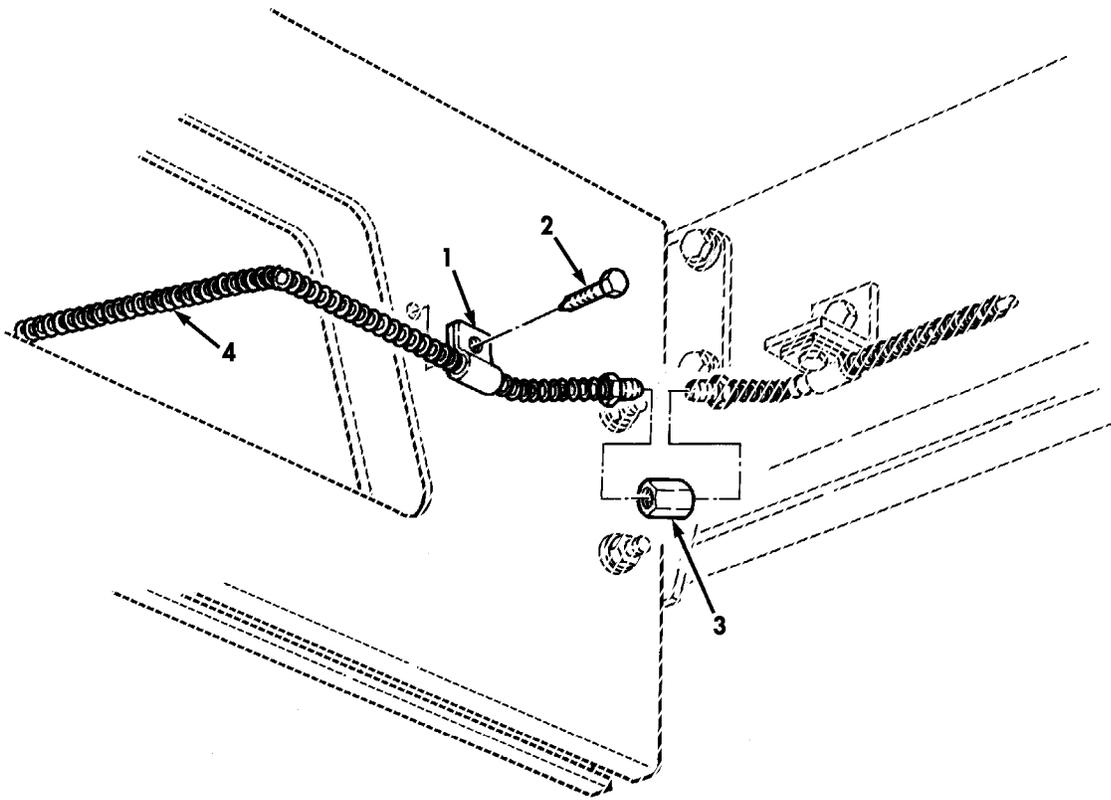
Figure 487C. Flexible Brake Line Kit.
