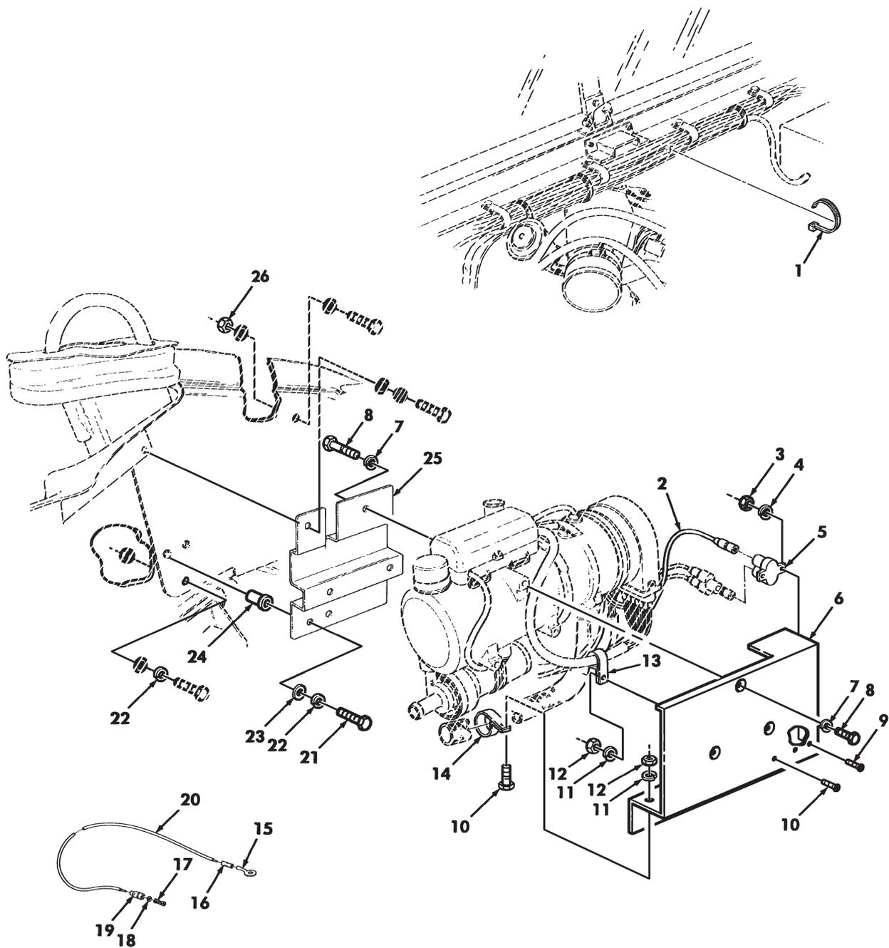
Figure 397B. Engine and Crew Compartment Heater Support Bracket, Heat Shield, and Mounting Hardware.
