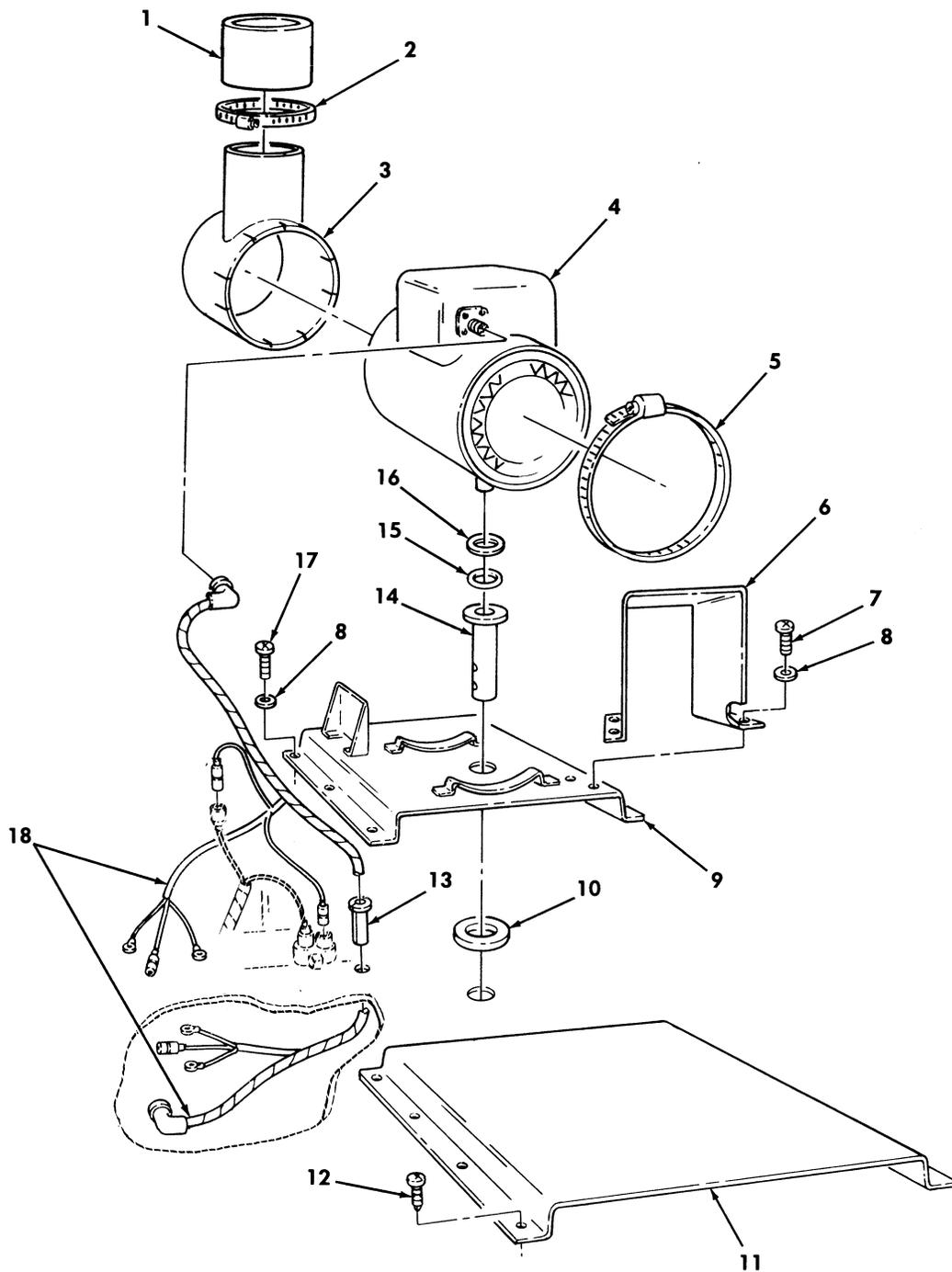
Figure 387. Winterization Kit, Heater and Exhaust Diverter Assembly.
