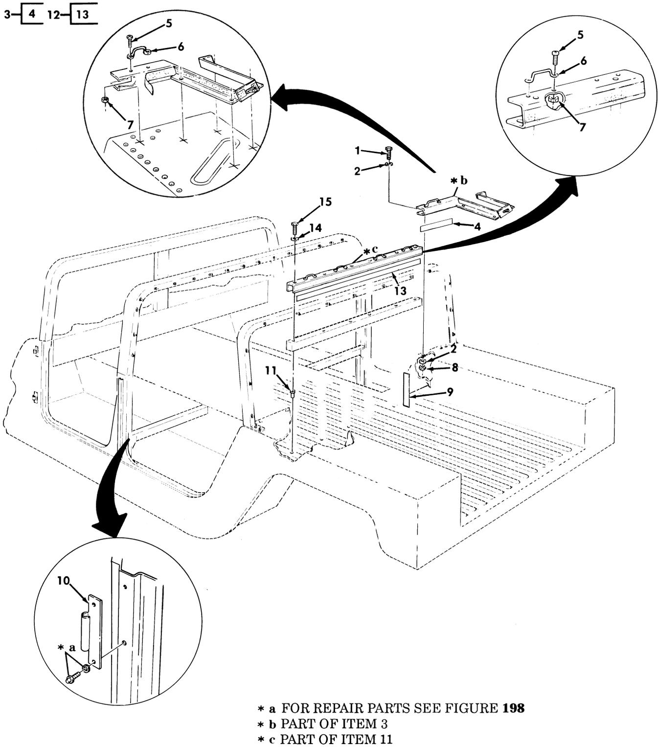
Figure 377. Arctic Kit, Door Hinges, and Curtain Channels.
