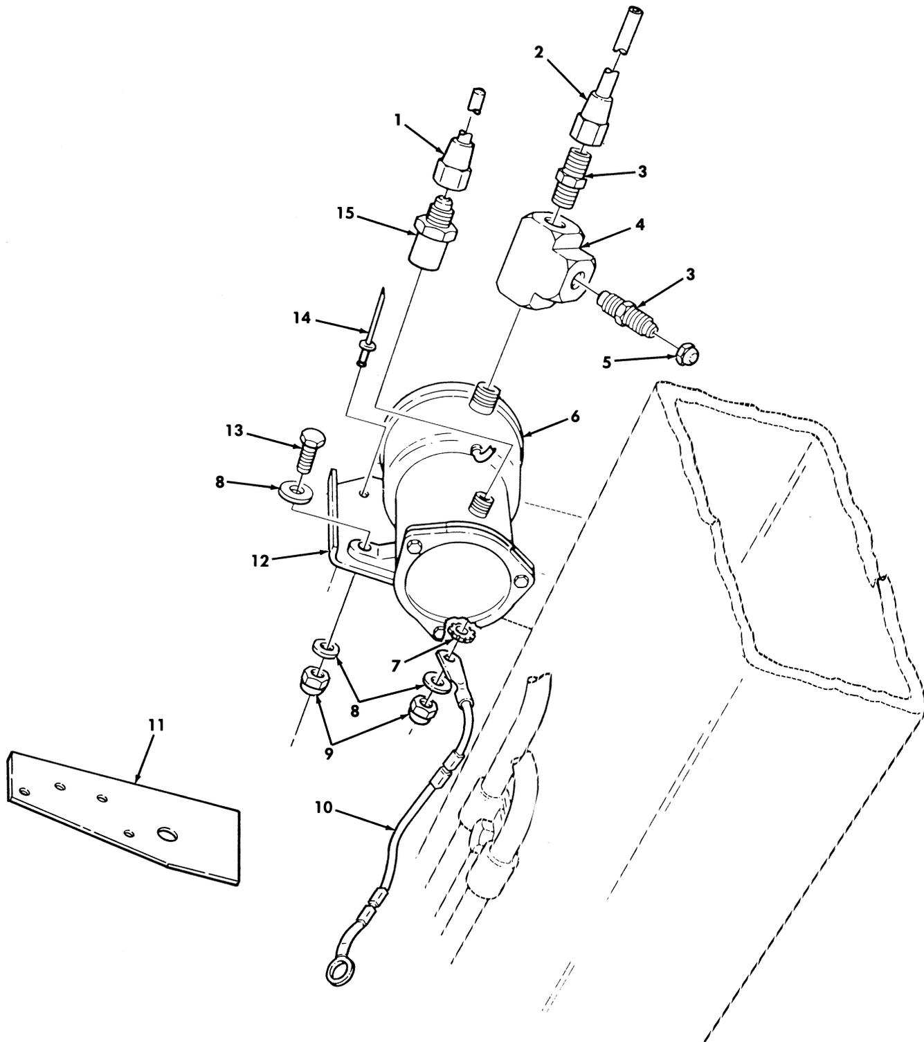
Figure 384. Winterization Kit, Fuel Pump, and Attaching Hardware.
