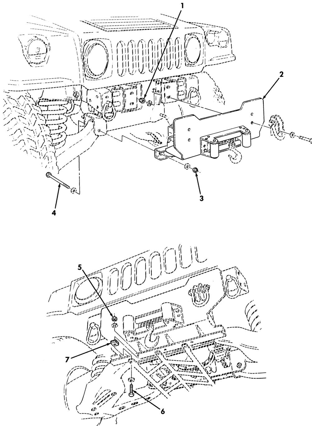
Figure 471. 10,500 Lb Hydraulic Winch Accessory Kit.
