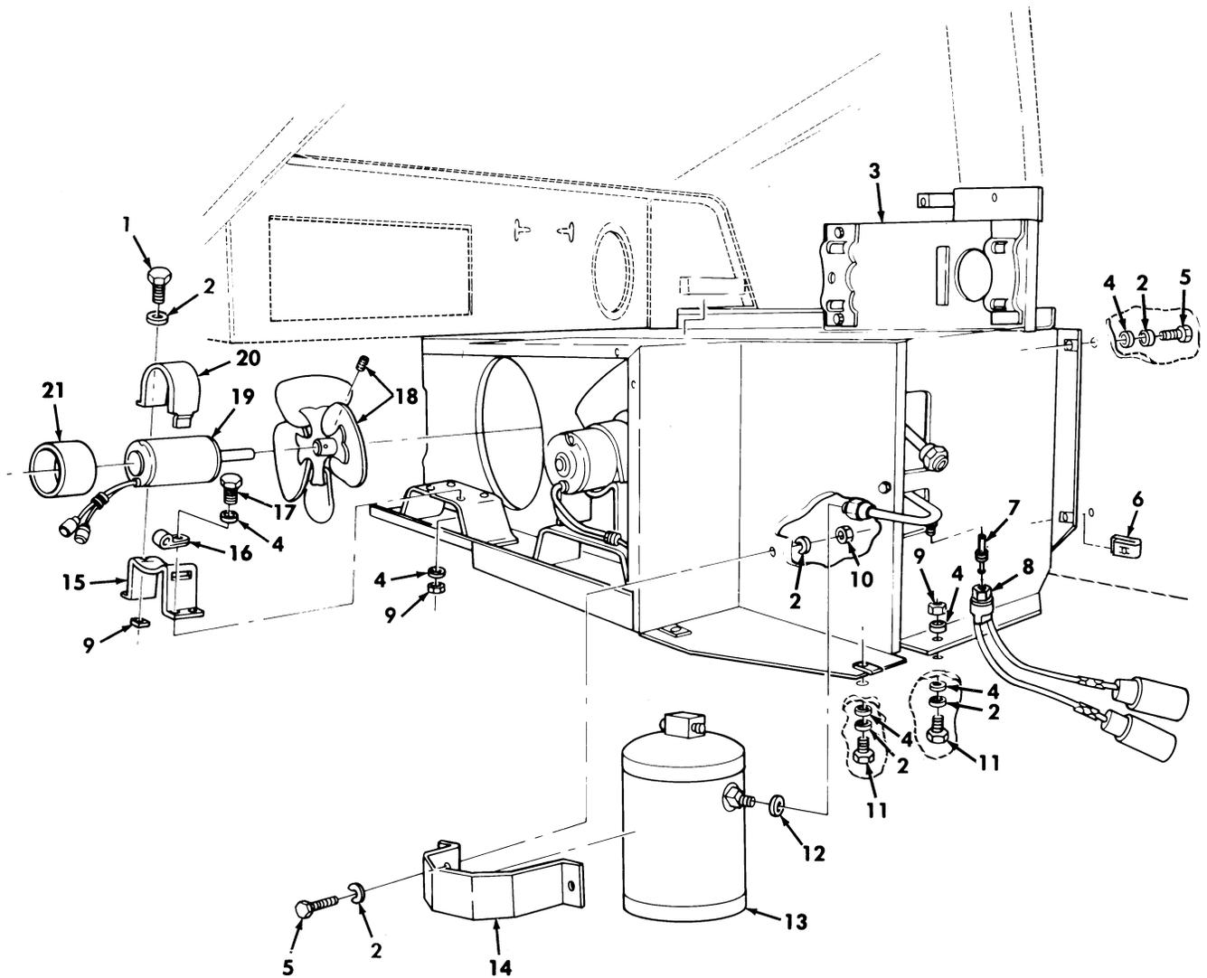
Figure 494. Heater and Air Conditioning Condenser, M997, M997A1, and M997A2 Ambulance.
