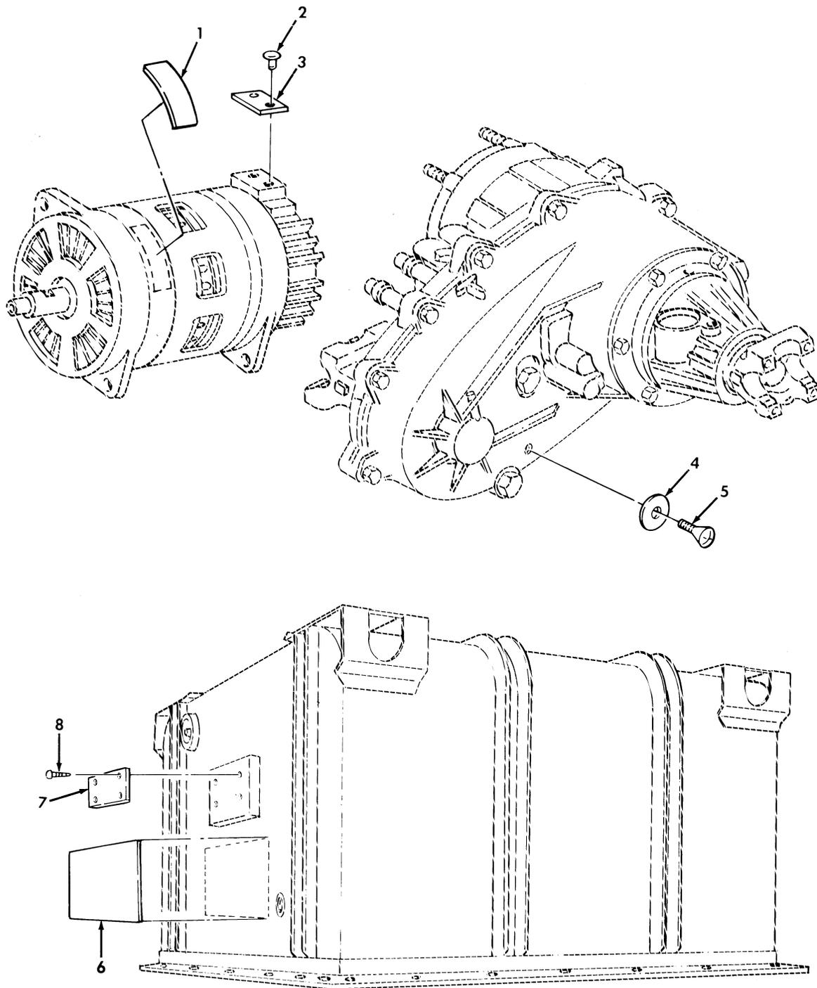
Figure 357. Data Plates, Generator, Transfer Case, and Engine Container.
