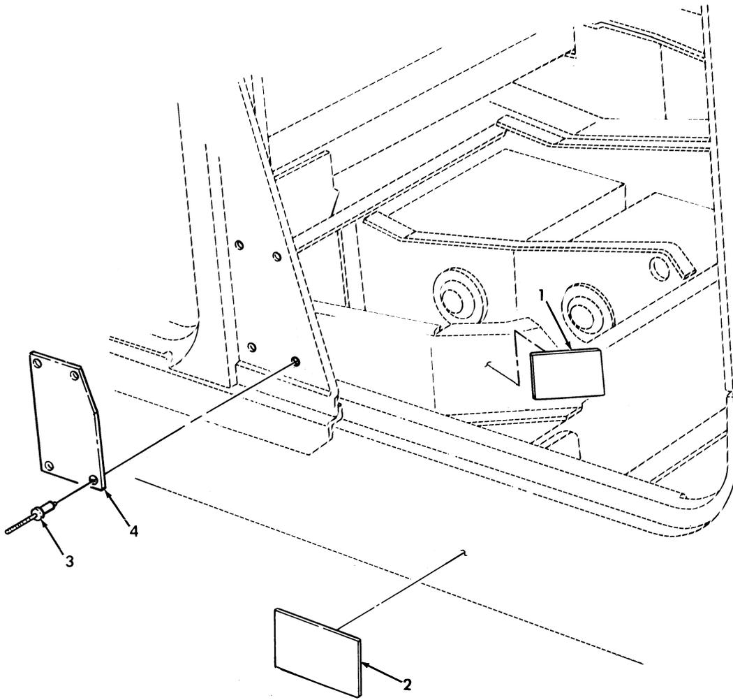
*Figure 355. Data Plates, Battery Cable and Slave Receptacle.*
