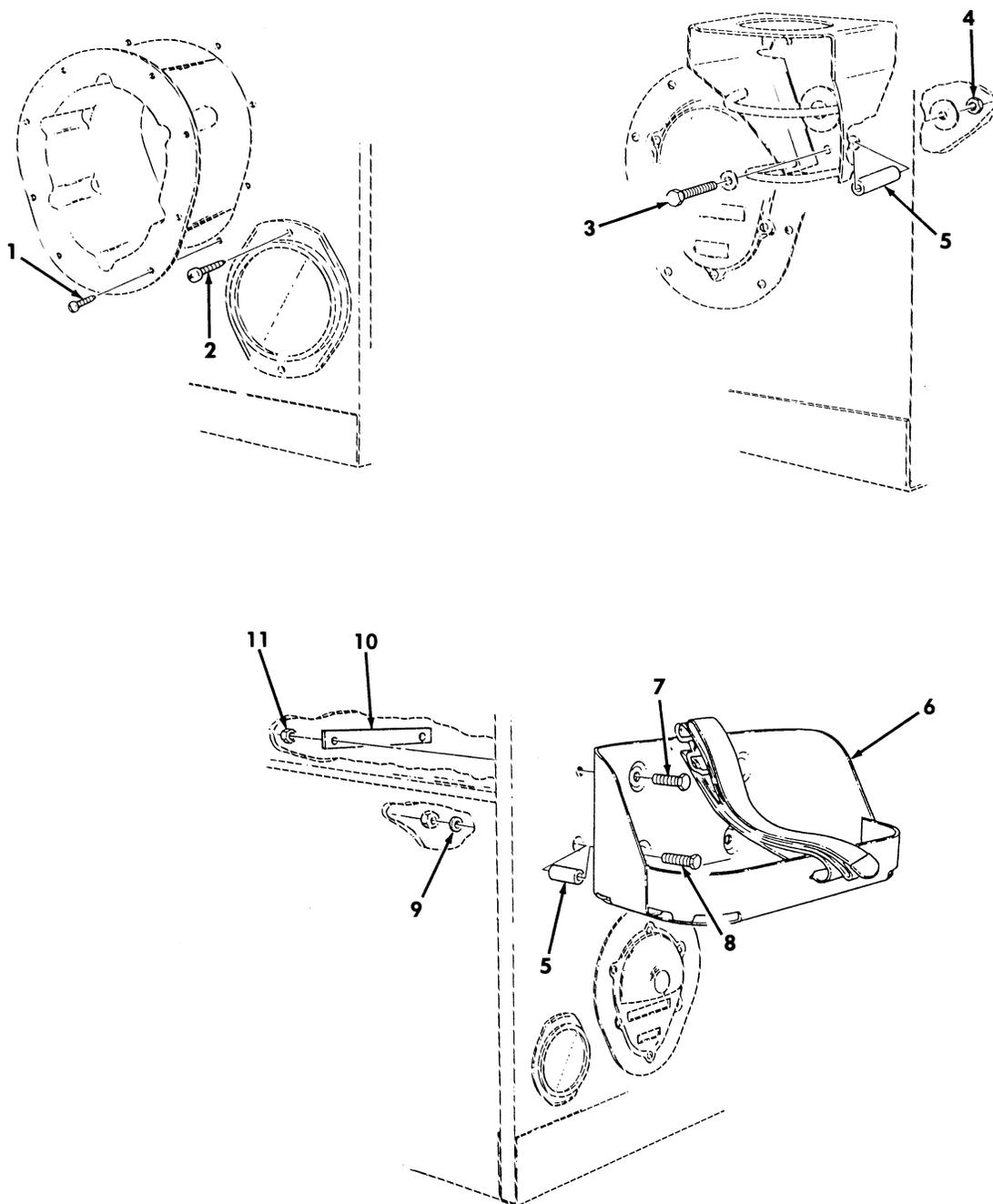
*Figure 392. Fuel Can Bracket, Antenna Mounting Bracket, and Composite Light Housing Mounting Hardware.*
