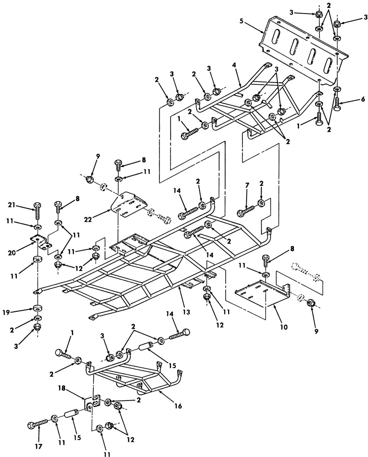
Figure 463. Underbody Protection Kit With and Without Winch.
