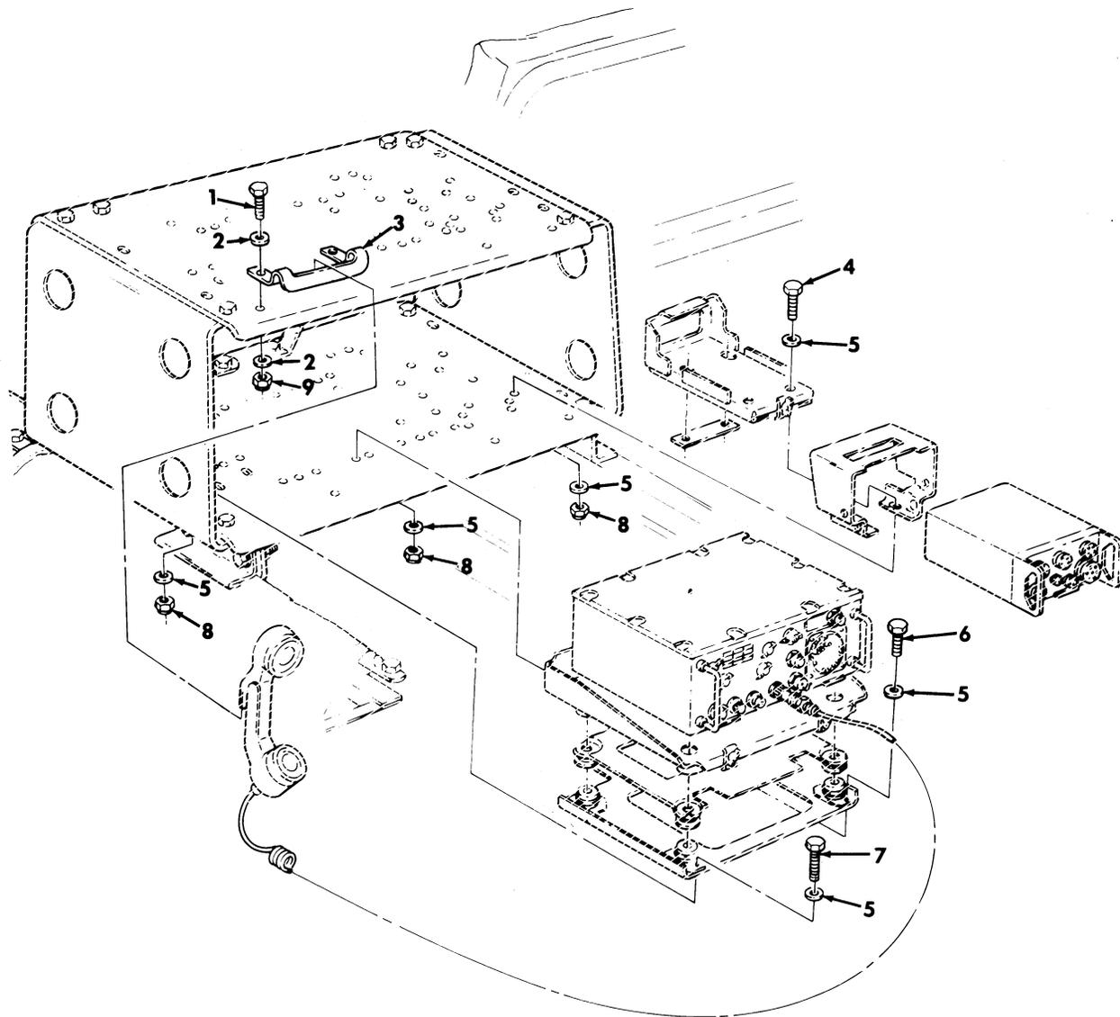
Figure 418. Communications Kit, Radio Rack Assembly Mounting Hardware, AN/VRC-46.
