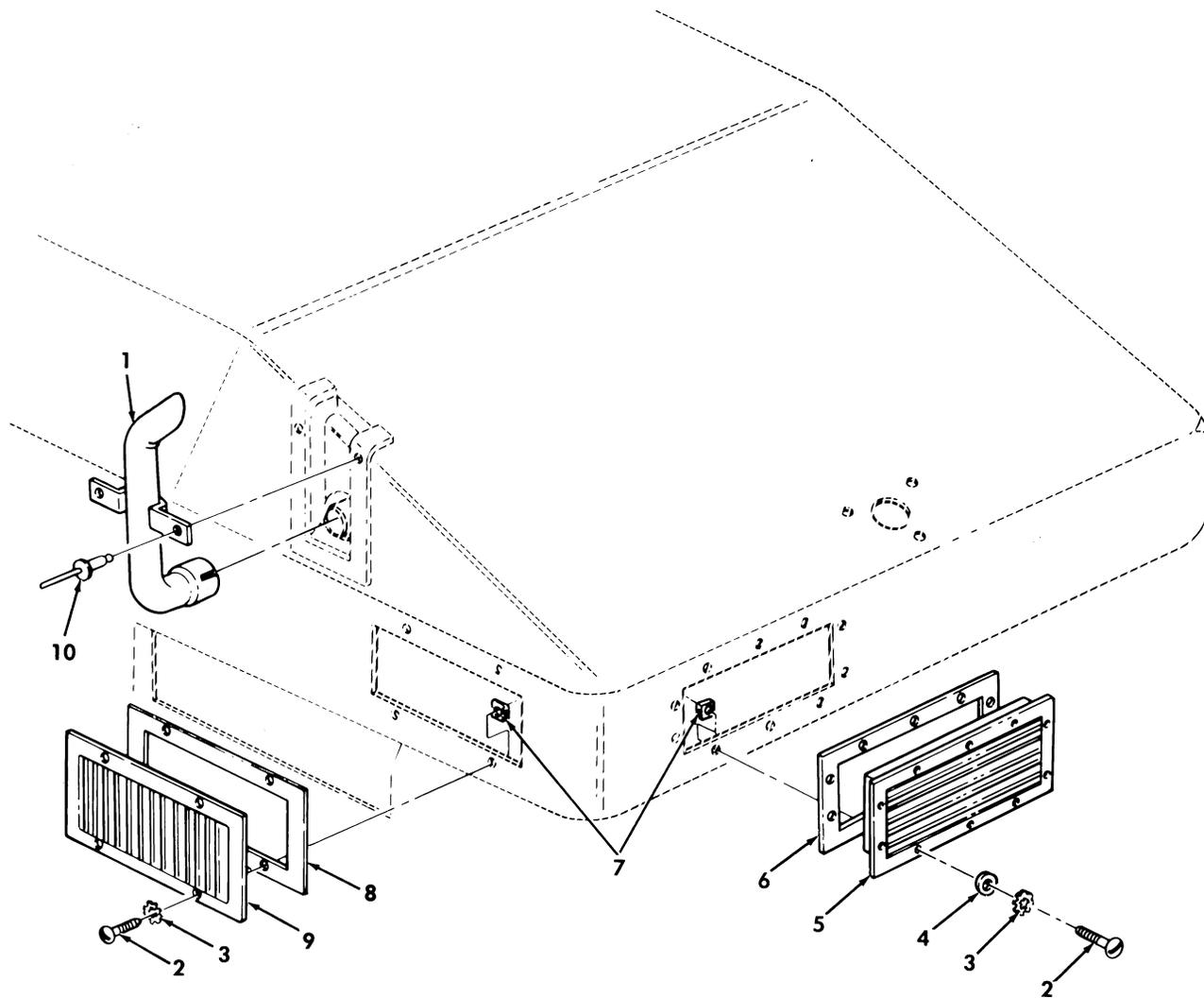
Figure 347. Heater Grille, Exhaust Pipe, and Mounting Hardware, M997, M997A1, and M997A2, Ambulance.
