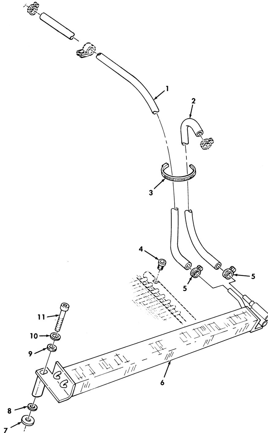
Figure 436. Power Steering Oil Cooler Kit.
