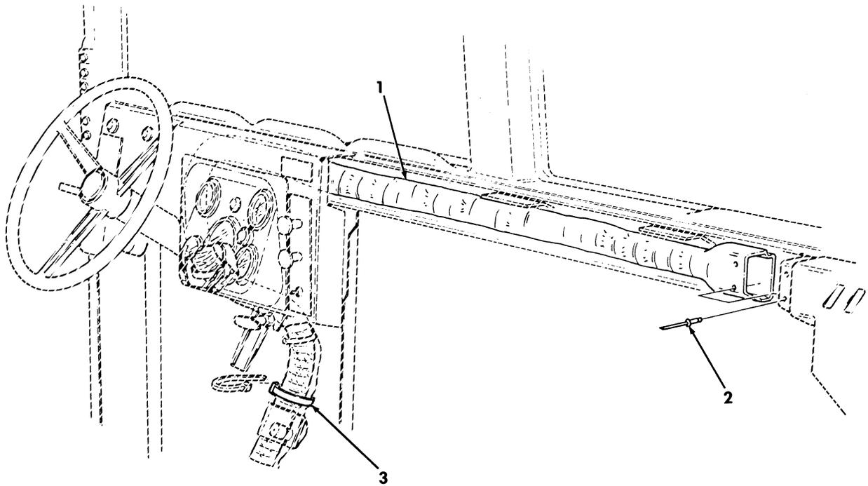
Figure 371. Arctic Kit, Heater Duct Assembly.
