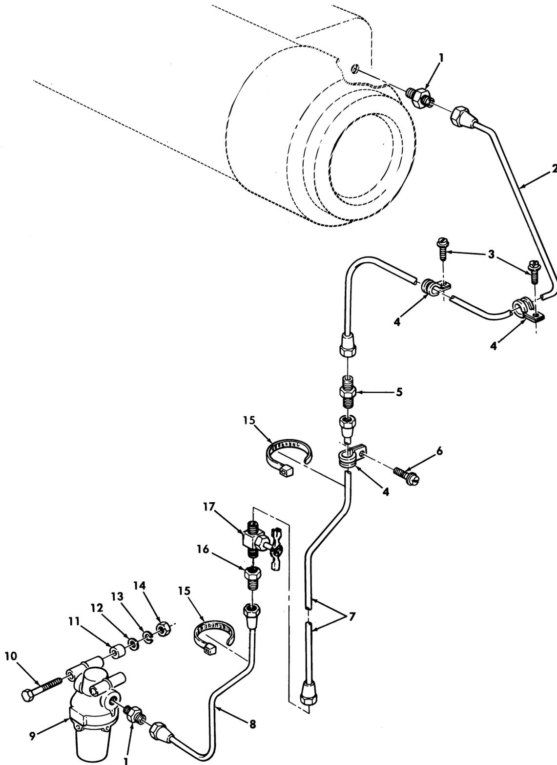
Figure 335. Fuel Lines, Personnel Heater to Fuel Filter, M996 and M996A1 Ambulance.
