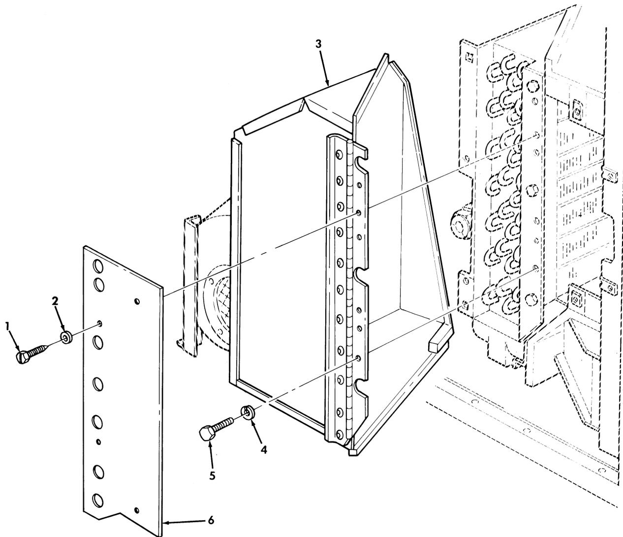
Figure 497. Evaporator Blower Motor Assembly Covers, M997, M997A1, and M997A2 Ambulance.
