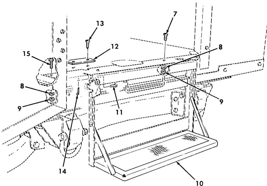
Figure 390. Step Assembly, Support Assembly, and Mounting Hardware.
