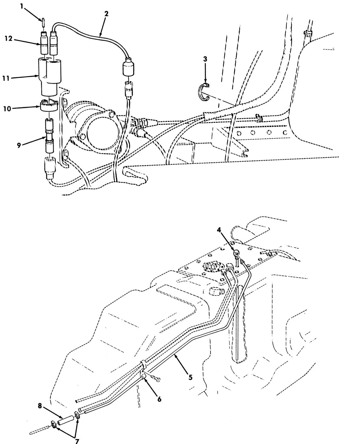
Figure 386. Winterization Kit, Fuel Line and Jumper Cable.
