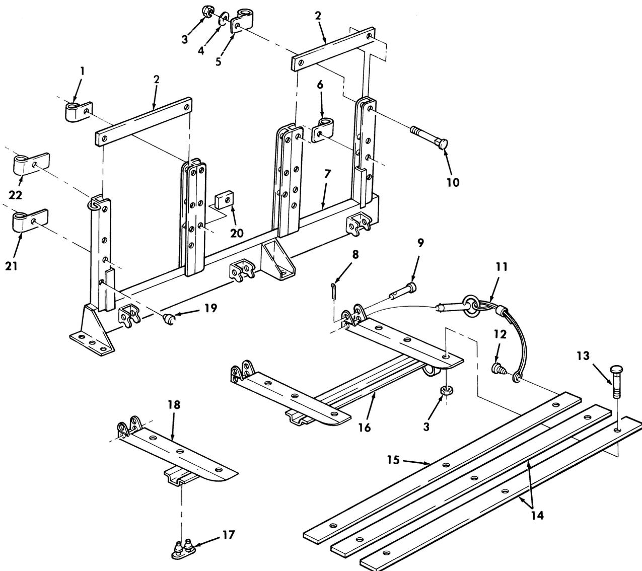
Figure 403. Troop Seat Assembly, Left and Right.
