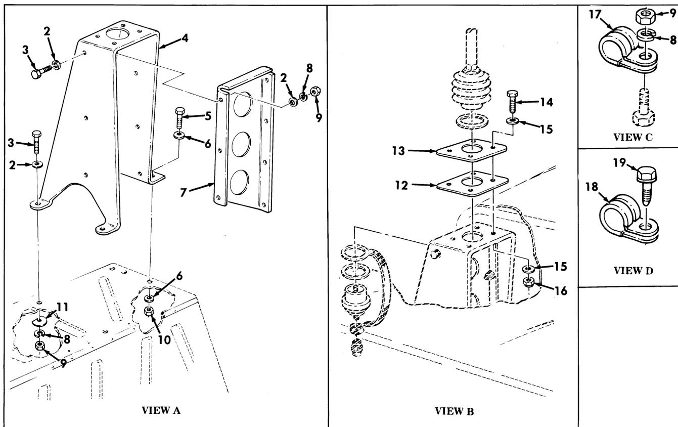
Figure 425. Communications Kit, Radio Cables, AN/VRC-47 and AN/VRC-48.
