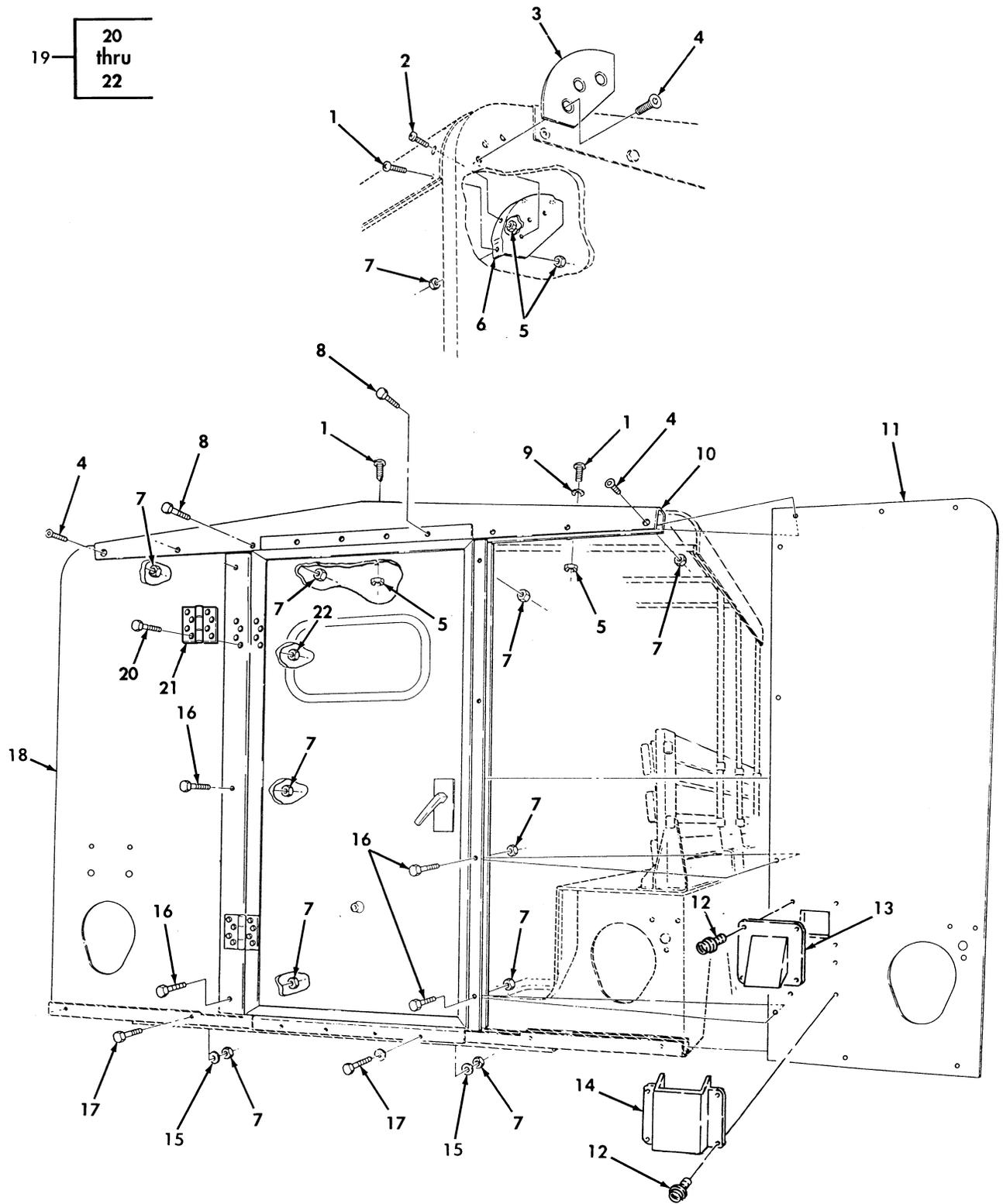
Figure 397. End Closures, Door Assembly, and Mounting Hardware.
