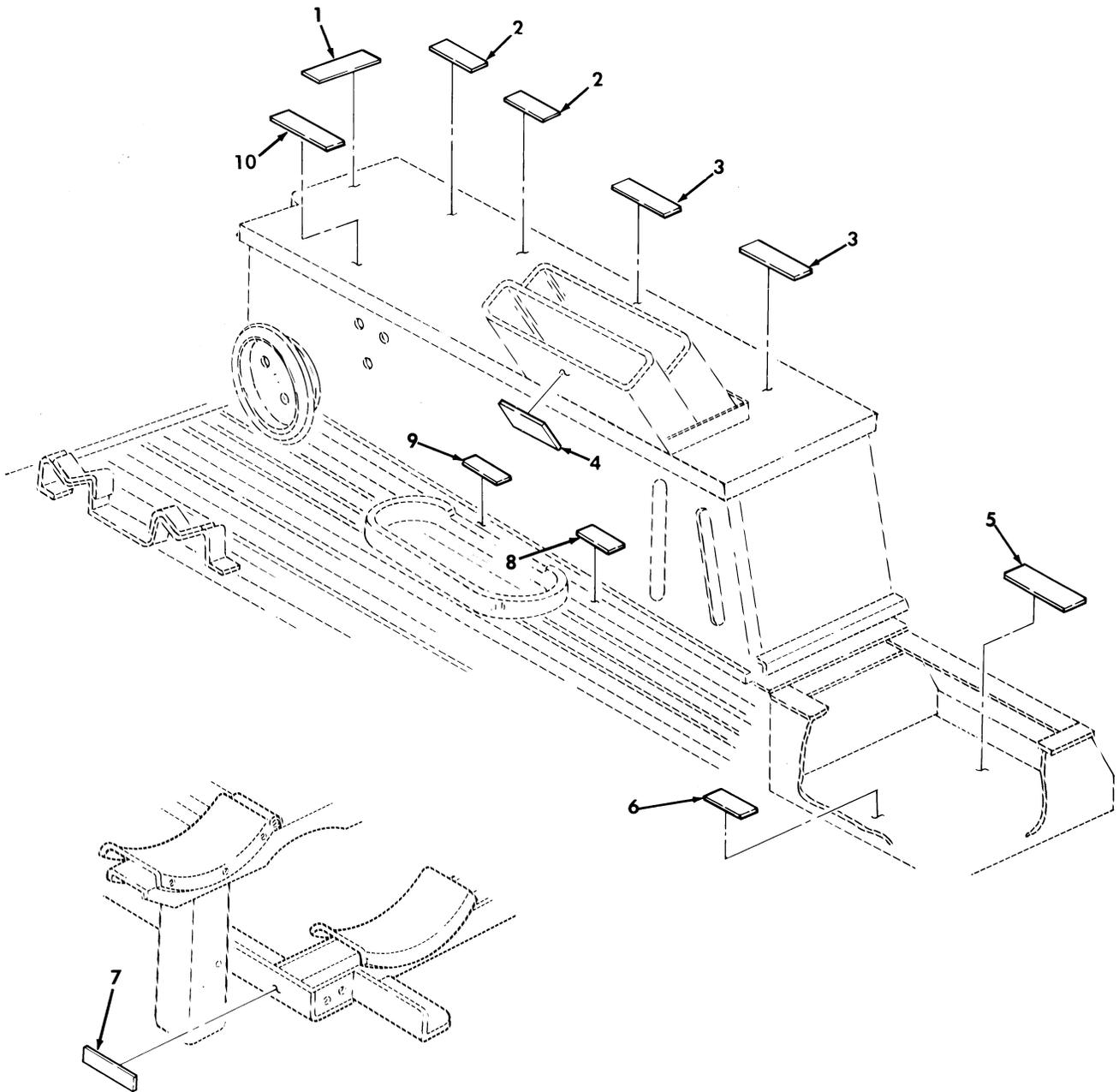
Figure 359. Data Plates, TOW Carrier.
