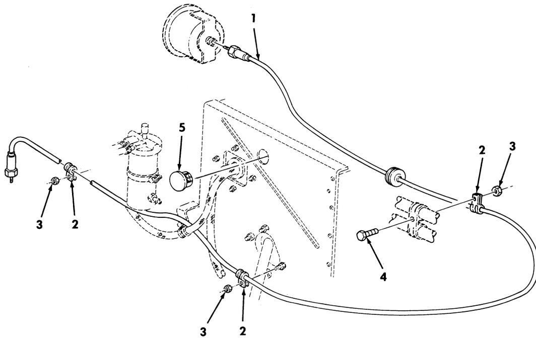
Figure 478. Speedometer Cable Assembly-400 AMP Alternator Kit.
