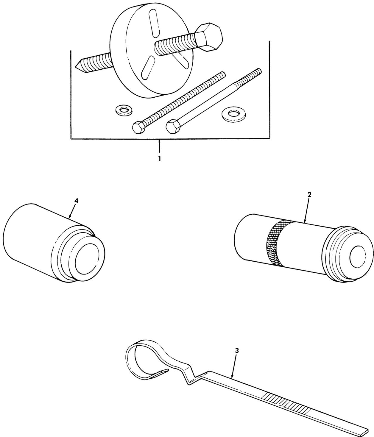
Figure 506. Special Tools, Air Conditioner Compressor.
