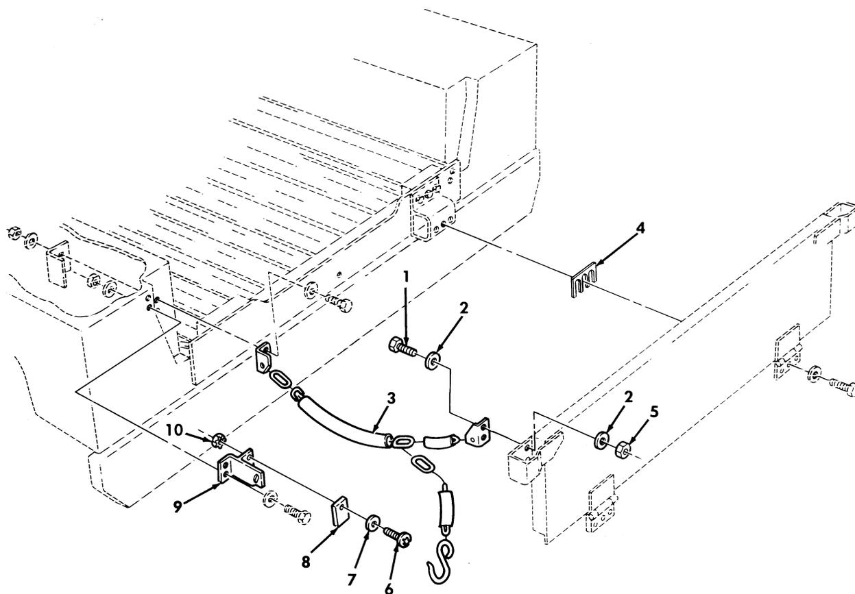
Figure 439. Kit, S250 Shelter Tailgate Mounting Components.
