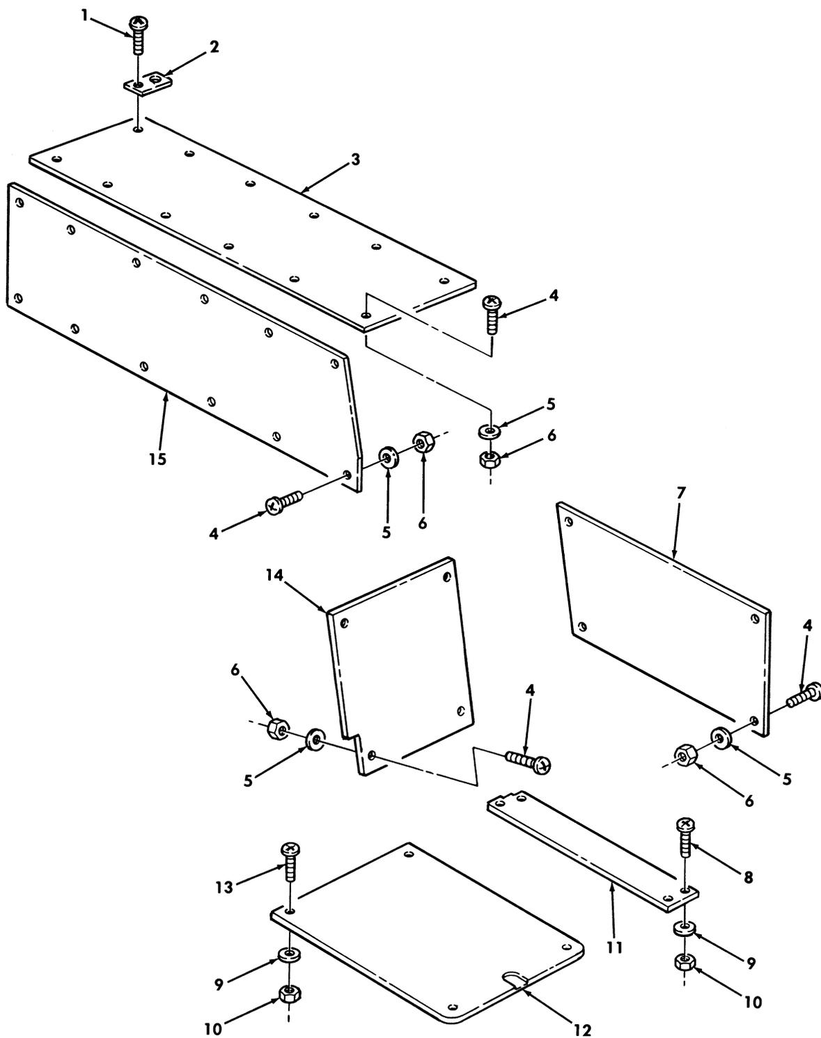
Figure 382. Two Door Seat and Floor Covers.
