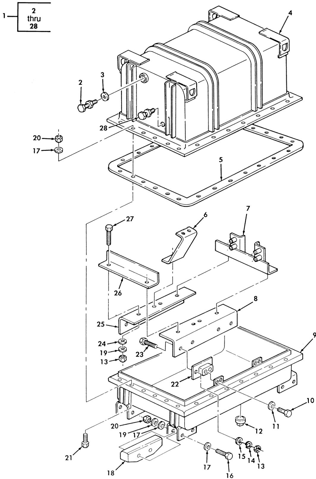
Figure 363. Engine Shipping Container Assembly.
