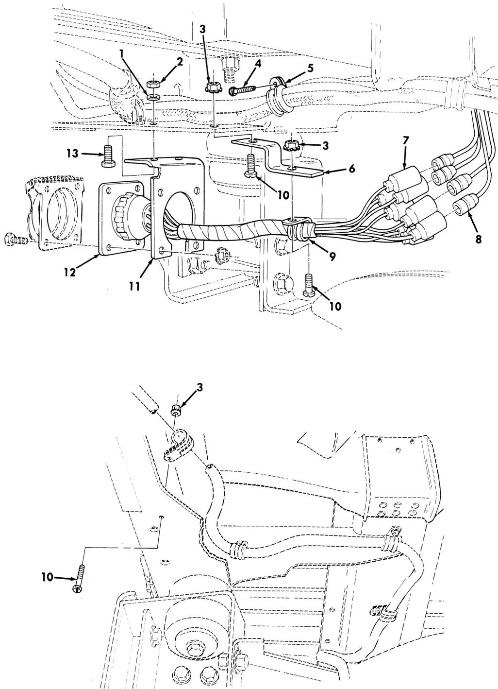
Figure 445. Kit, Prime Mover, Lt. Howitzer, 105 MM L119, Trailer Receptacle and Body Wiring Harness.
