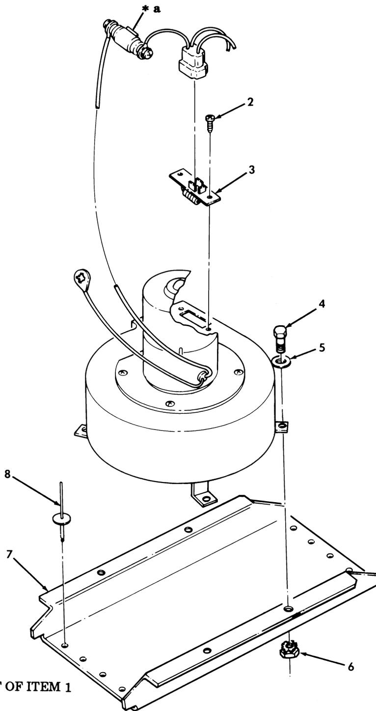
Figure 342. Heater Blower Assembly, M996 and M996A1 Ambulance.
