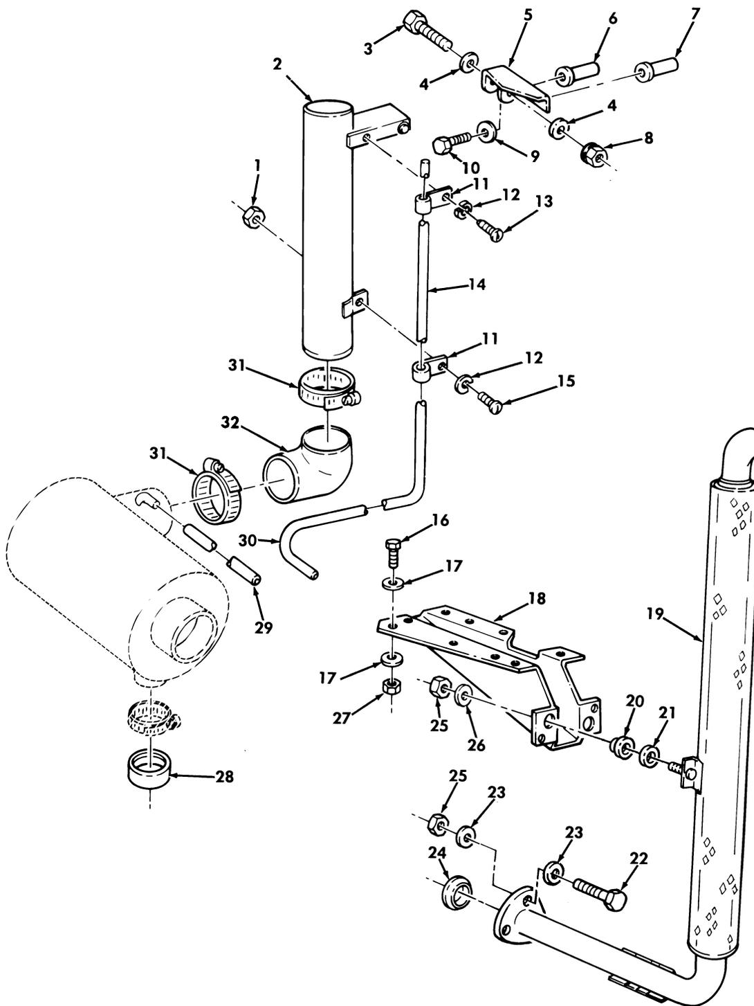
Figure 398. Deep Water Fording Kit, Intake and Exhaust Systems.
